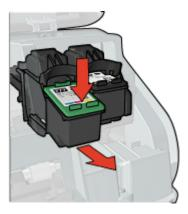
**6.** Remove the replacement print cartridge from its packaging and carefully remove the plastic tape. Hold the print cartridge so that the copper strips are on the bottom and facing toward the printer.
