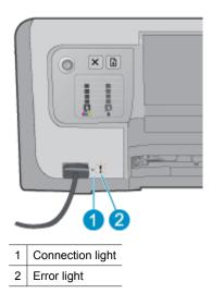
When the camera is connected correctly, the Connection light is illuminated. The Connection light blinks green when printing from the camera. If the camera is not set to the correct mode for downloading photos, the Error light flashes.
