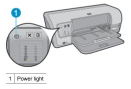
If the Power light is flashing, the printer is preparing to print. The light stops flashing when the printer has received all data.
