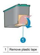
△ CAUTION: Do not touch the print cartridge ink nozzles or copper contacts. Touching these parts will result in clogs, ink failure, and bad electrical connections. Do not remove the copper strips. They are required electrical contacts.
