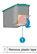
△ CAUTION: Do not touch the print cartridge ink nozzles or copper contacts. Touching these parts will result in clogs, ink failure, and bad electrical connections. Do not remove the copper strips. They are required electrical contacts.
