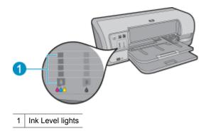
The lnk Level lights show ink level information for each print cartridge, four for the tri-color cartridge and four for the black/photo cartridge.
