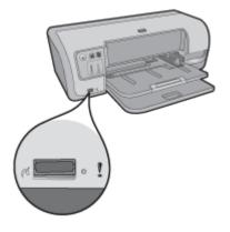
In order to transfer photos from your digital camera to the computer for printing, using the front USB port, you need a USB cable that is compatible with your camera. HP recommends that you use a cable that is less than 3 meters long.
