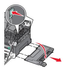
Press the green levers on each side of the waste toner bottle, and then remove it.
