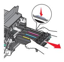
**8** Remove the used developer unit.
