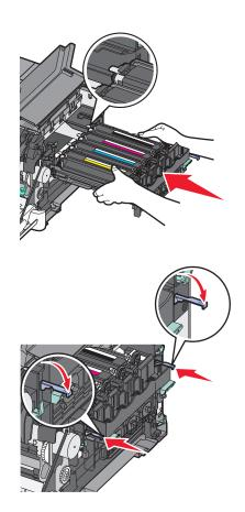
**16** Rotate the blue levers down until the imaging kit drops into place.
