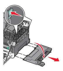
**5** Press the green levers on each side of the waste toner bottle, and then remove it.
