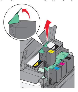
**5** Align the new toner cartridge, and then press down until it is all the way into the slot.
