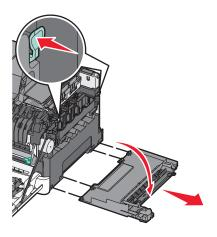
Press the green levers on each side of the waste toner bottle, and remove it.
