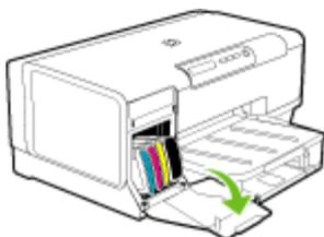
2. Remove the ink cartridge that requires replacement by grasping it between your thumb and forefinger and pulling it firmly toward you.
