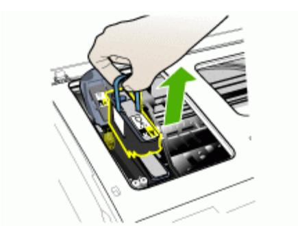
5. Place the printheads in an airtight plastic container so they will not dry out, and put them aside. Do not send them with the device unless the HP customer support call agent instructs you to.
