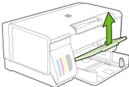
2. Insert the media print-side down along the right of the tray. Make sure the stack of media aligns with the right and back edges of the tray, and does not exceed the line marking in the tray.
