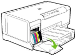
3. Remove the ink cartridges from their slots by grasping each between your thumb and forefinger and pulling it firmly toward you.
