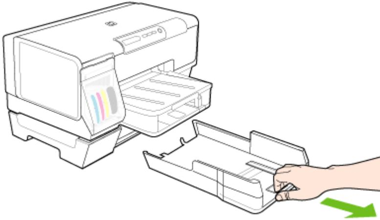
2. Insert the paper print-side down along the right of the tray. Make sure the stack of paper aligns with the right and back edges of the tray, and does not exceed the line marking in the tray.
