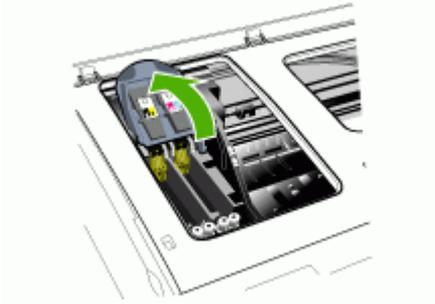
4. Lift the handle of the printhead you want to replace and pull the printhead out of its slot.
