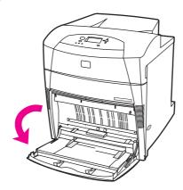
2. Load up to 20 envelopes in the center of Tray 1 with the side to be printed on facing down, top on the left, and the short edge toward the printer. Slide the envelopes into the printer as far as they will go without forcing them.
