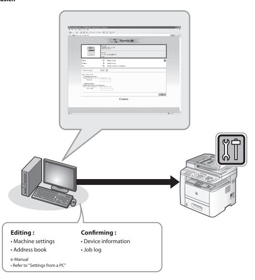
By using Remote UI, you can set and confirm following functions.
