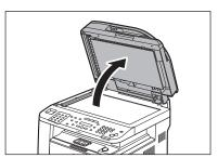
Clean the platen glass and the underside of the ADF with a cloth dampened with water. Then, wipe the area with a soft, dry cloth.
