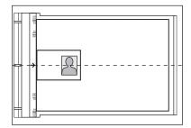
Align the center of a card with the arrow mark.
