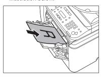
The display for specifying the paper size and type appears if <MP TRAY STD SET> is set to <OFF>. For details, see "Setting Paper Size and Type," on p. 2-17.
