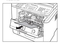
Align the toner cartridge to the guides in the machine and slide the cartridge completely into the machine until it stops.
