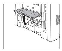
Open and close the front cover to reset the machine.
