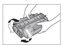
Align the toner cartridge to the guides in the machine and slide the cartridge completely into the machine until it stops.
