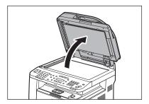
Clean the ADF scanning area (on the left side of the platen glass (A)) with a cloth dampened with water. Then wipe the area with a soft, dry cloth.
