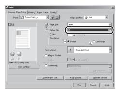
The document is scaled automatically according to the settings made in [Page Size] and [Output Size].
