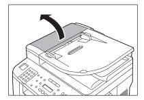
Clean the rollers (A) inside the ADF with a cloth dampened with water. Then wipe the area with a soft, dry cloth.
