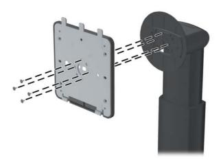
5. Remove four screws to separate the mounting plate from its cover:
