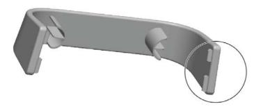
1. To remove the bar, first pull one end of the bar away from the pedestal (1). When it is free, the bar can be removed (2).
