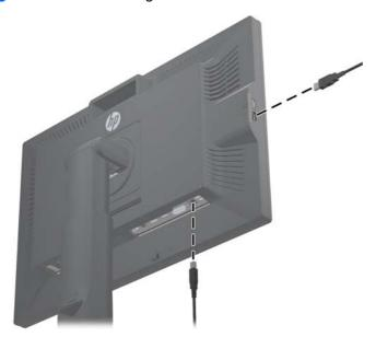
5. Connect one end of the power cable to the AC power connector on the back of the monitor, and the other end to an electrical wall outlet.
