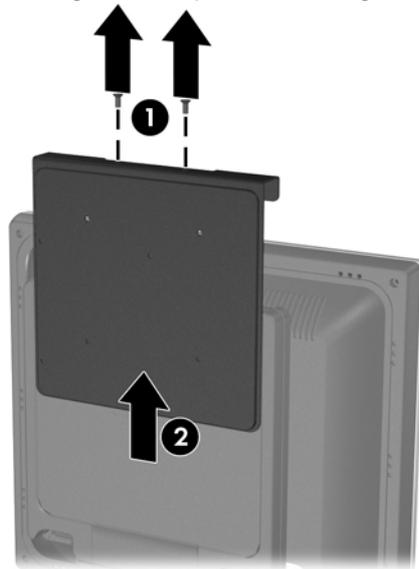
2. Remove the HP logo panel from the right side of the Thin Client to access the screw holes for the computer mounting bracket.
