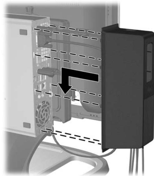
7. Slide the power supply tray out from the base of the stand (1) and place the USDT power supply into the tray (2). Route any loose cables through the cables guides on the sides of the tray (3).
