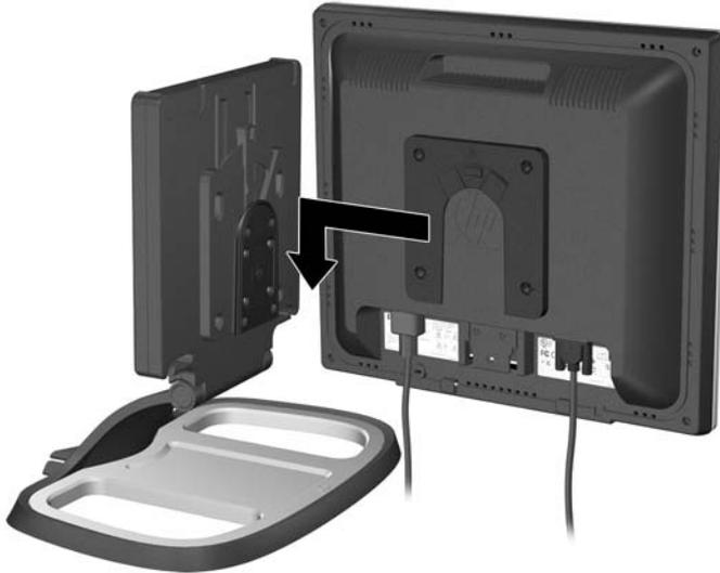
3. Route the monitor VGA and power cables through the cable guides at the bottom corners of the mounting panel.
