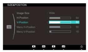
4 Adjust the V-Position using the [▲/▼] button.
