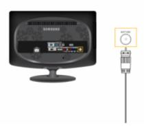
1. Connect the CATV cable or TV antenna cable to the "ANT IN" port on the rear side of the monitor.
