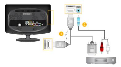
Onnect the DVI output terminal of a digital output device to the [HDMI IN1] or [HDMI IN2] terminal of the monitor using a DVI to HDMI cable.
