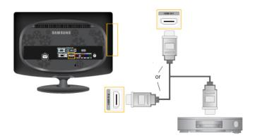
Input devices such as digital DVD are connected to the [HDMI IN1] or [HDMI IN2] terminal of the monitor using the HDMI cable. When all the connections are completed, connect the power cords for the monitor and DVD(or the device connected to the digital output terminal).
