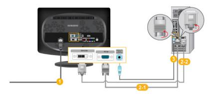
Oonnect the power cord for your monitor to the POWER port on the back of the monitor.
