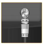
Connect the CATV cable or TV antenna cable to the "ANT IN" port on the rear side of the product. Make sure to use a TV antenna cable (sold separately) as the antenna cable.
