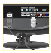
Fix the cables using the holding ring, as shown in the figure.
