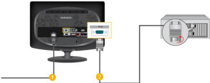
Onnect the power cord for your monitor to the POWER port on the back of the monitor.
