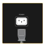
Connect the power cord for your monitor to the *POWER* port on the back of the product.
