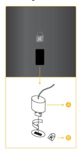
The Kensington Lock is a device used to physically fix the system when using it in a public place. The locking device has to be purchased separately. The appearance and locking method may differ from the illustration depending on the manufacturer. Refer to the manual provided with the Kensington Lock for proper use. The locking device has to be purchased separately.
