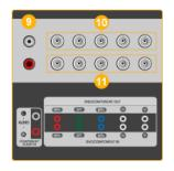
9 COMPONENT AUDIO IN [L-AUDIO-R] (Component Audio Connection Terminal (Input))
