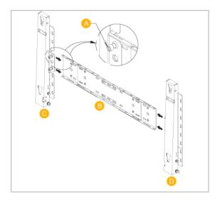
There are two hinges(left and right). Use the correct one.
