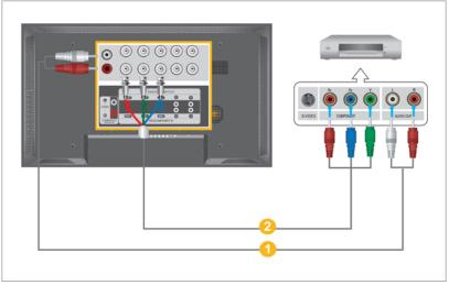
Connect a set of audio cables between the COMPONENT AUDIO IN [L-AUDIO-R] on the LCD Display and the AUDIO OUT jacks on the DVD player.
