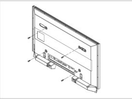
2. Insert the screw B into the plastic hanger.
