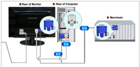
Connect the power cord for your monitor to the power port on the back of the monitor.
