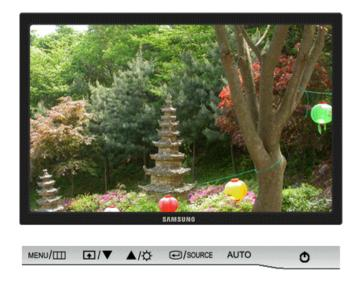
When OSD is not on the screen, push the **Brightness** ( ) button to adjust brightness.
