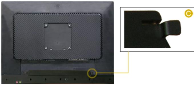
For removal, push and lift up part (C) towards the inside and remove it. Failing to do so may damage the unit.
