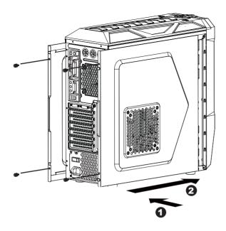
Make sure all necessary cables and wires are connected, then reinstall side panels and secure with screws.
