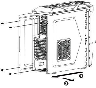
Unscrew to remove left and right panels.
