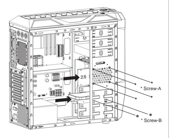
Put the 3.5"/2.5" HDD/SSD onto the HDD tray then secure with screws.
