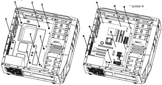
Step 1- Install motherboard stand-offs according to your motherboard's form factor.
