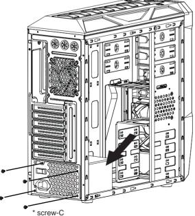
Place the power supply from the left side into the chassis and secure with screws.
