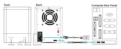
• Power ON/OFF: Switch the power button located in the back to power on/off.
