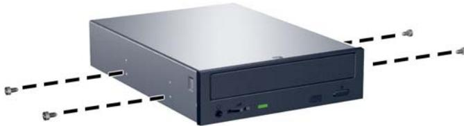
5. Position the guide screws on the drive into the J-slots in the drive bay. Then slide the drive toward the front of the computer until it locks into place.
