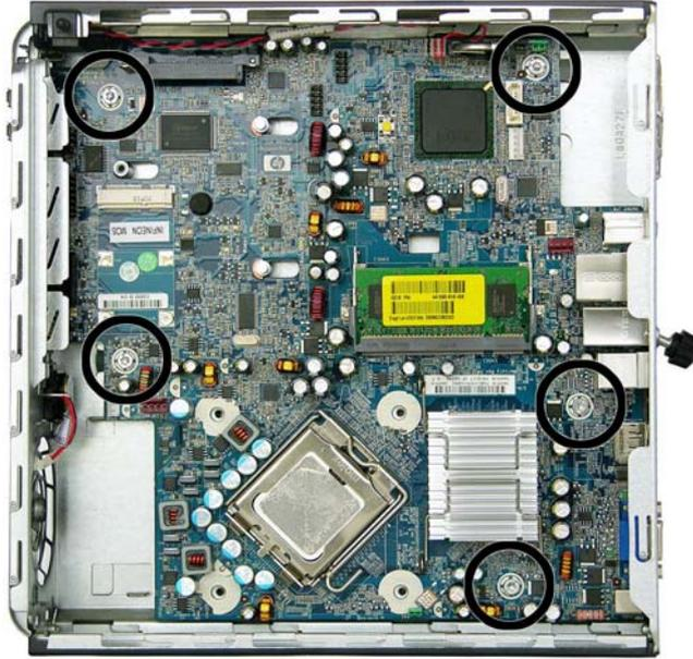
11. Slide system board toward the front of the unit until the rear connectors are clear of their slots in the chassis.
