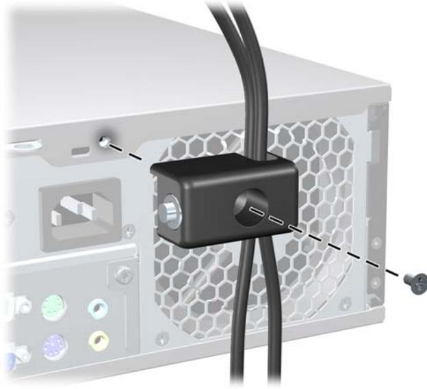
4. Insert the plug end of the security cable into the lock (1) and push the button in (2) to engage the lock. Use the key provided to disengage the lock.
