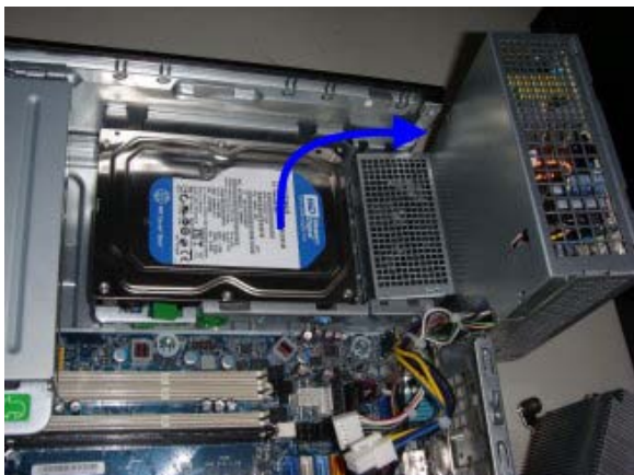
Figure21: Remove PSU from Chassis
