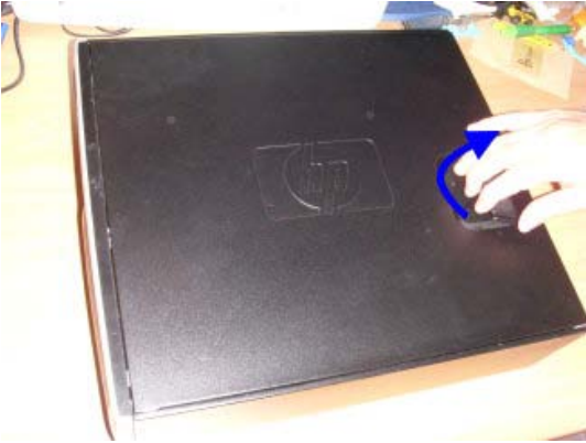
Figure 3: Pull 3 retaining clips on the bezel top side
