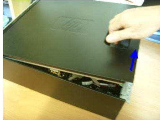
Figure 2: Rise access panck Press front panel clip
