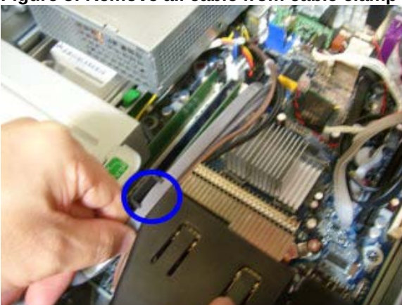
Figure 5: Remove all cable from cable clamp
