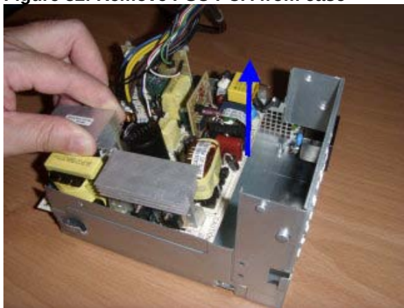
Figure 32: Remove PSU PCA from case
