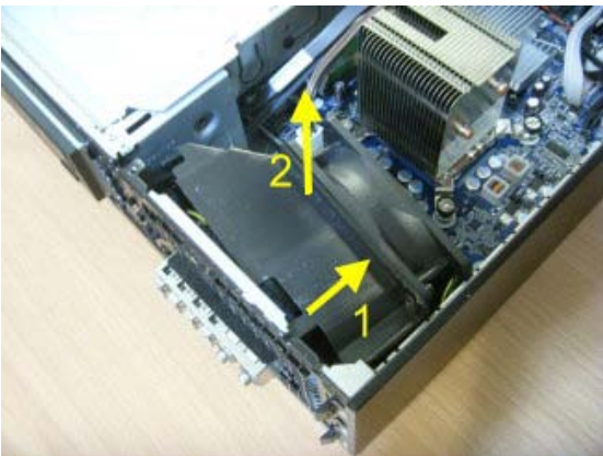
Figure 9 : Remove fan and fan holder from chassis
