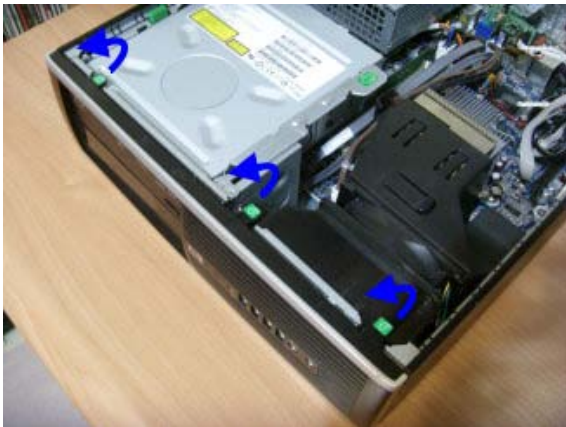
Figure 5: Remove all cable from cable clamp
