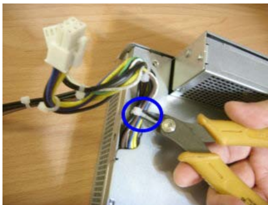
Figure 28: Remove PSU the top of case
