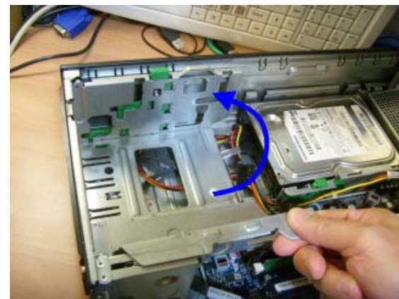
Figure 18: Rotage ODD cable to vertical
