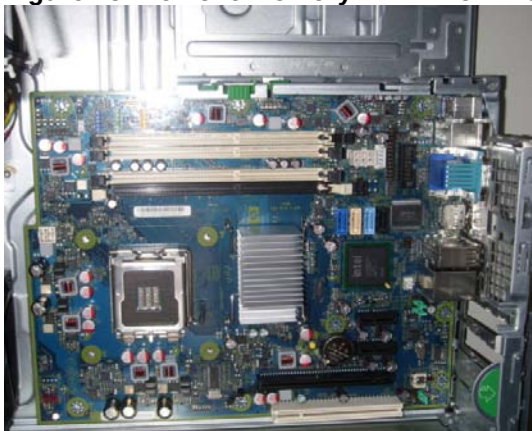
Figure 15 :Remove Memory DIMM from PCA
