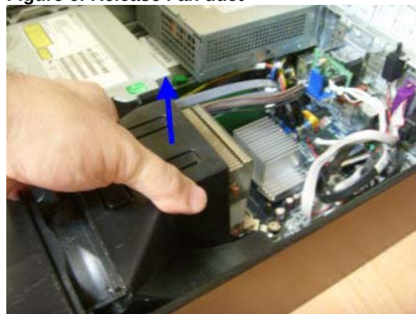
Figure 6: Release Fan duct
