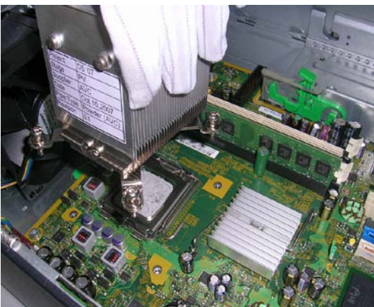
Figure 11: Remove Heat sink from PCA
