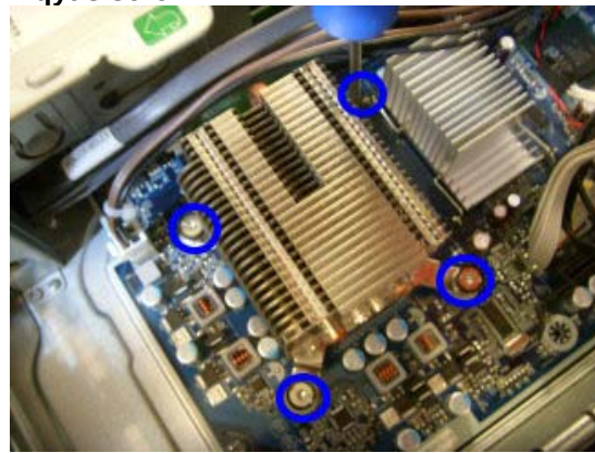
Figure 10 : Wresting screw with screw driver release 4 qyt's screw
