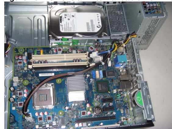
Figure 16: Remove all internal cable from PCA
