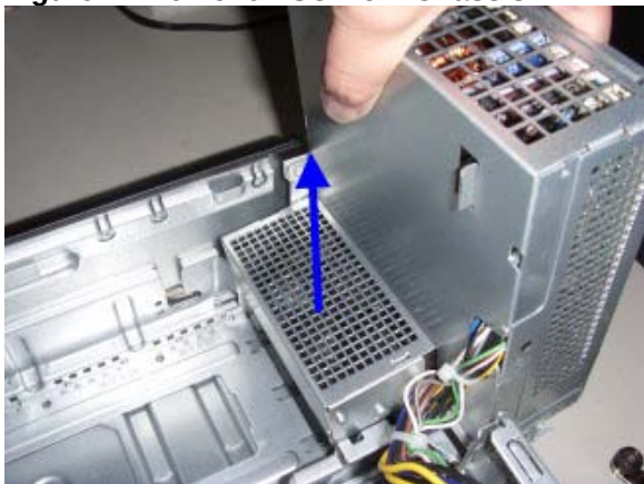
Figure21: Remove PSU from Chassis
