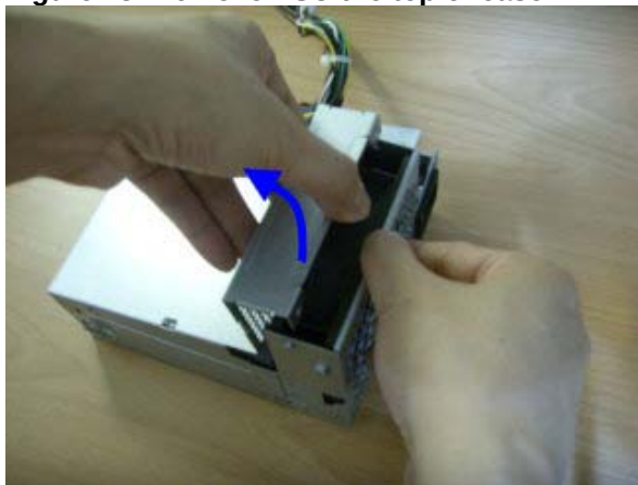
Figure 28: Remove PSU the top of case
