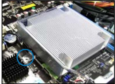
3. Replace the screw and secure the airduct onto the motherboard.
