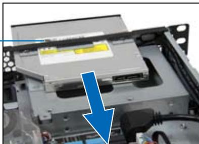
2. Align the screw hole of the ODD bracket with the screw hole on the chassis. Secure the ODD with a screw.
