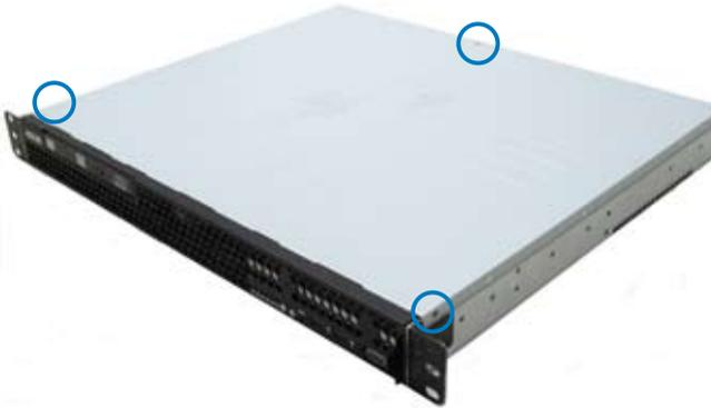
2. Firmly hold the cover and slide it toward the rear panel for about half an inch until it is disengaged from the chassis.
