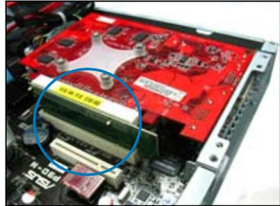
5. Secure the expansion card to the bracket with a screw.
