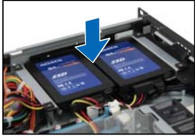
16. Secure the 2.5-inch SSD and SSD drive tray assembly to the HDD bay 1 using the screws removed in step 3.
