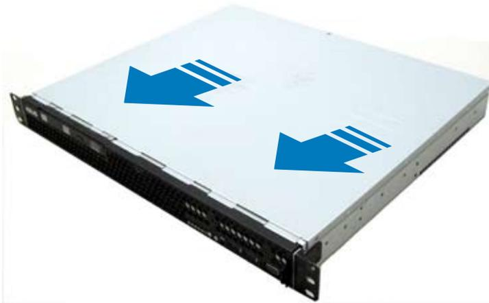
3. Secure the cover with three screws.
