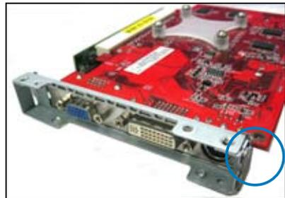
6. Secure the assembly to the chassis with a screw.
