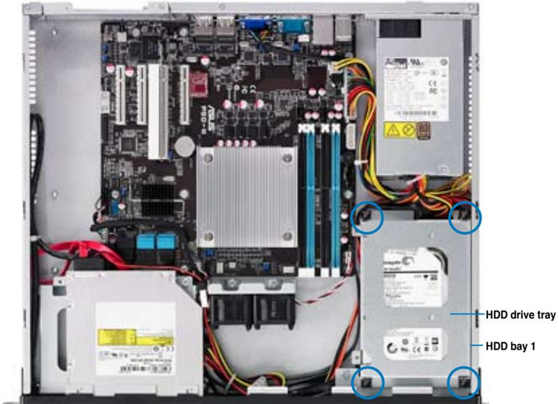
4. Remove the HDD drive tray and 3.5-inch SATA HDD assembly.
