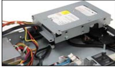
7. Place and orient the HDD tray and 3.5-inch SATA HDD assembly in such a way that the SATA cable and power connector is aligned towards the rear (as shown).
