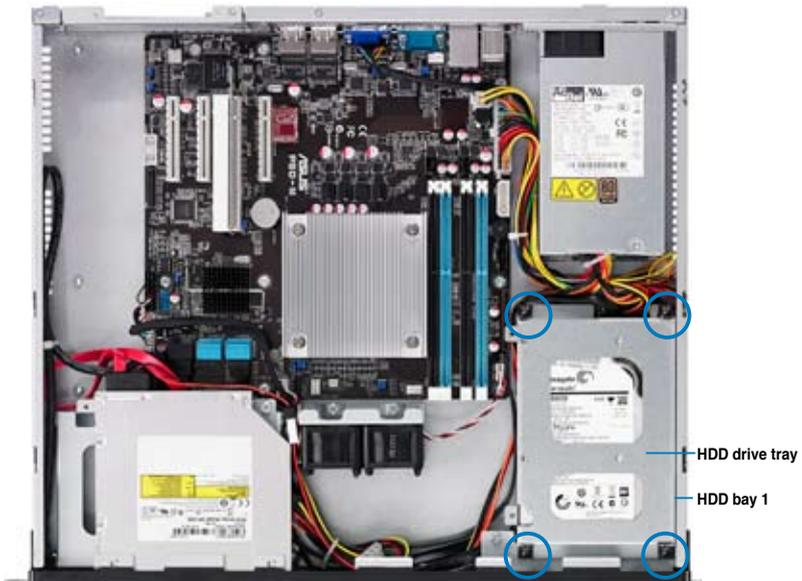
4. Prepare a 3.5-inch Serial ATA HDD and the set of bundled screws.
