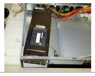
8. Install power supply housing. Place and tilt the power supply housing inside the chassis with slanted angle to let the housing get through the opening of chassis rear panel
