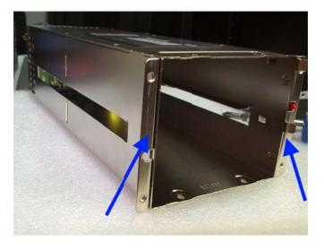
3. Remove power supply's brackets from both sides
