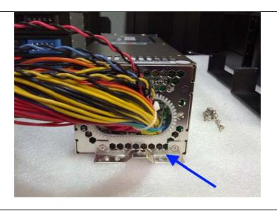
6. Install power supply rear bracket comes with power supply
