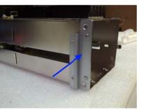
5. Install power supply brackets come with chassis
