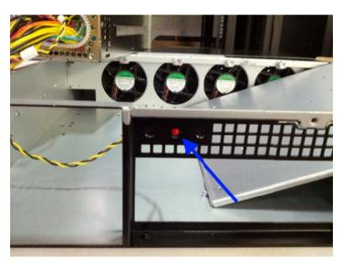
7. Install power supply reset button to the chassis
