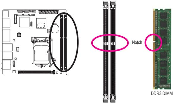
A DDR3 memory module has a notch, so it can only fit in one direction. Follow the steps below to correctly install your memory modules in the memory sockets.
