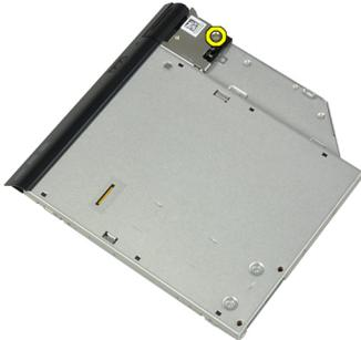
6. Push the optical-drive latch forward and remove it from the optical-drive assembly.
