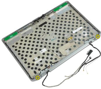
6. Remove the display hinges from the display assembly.
