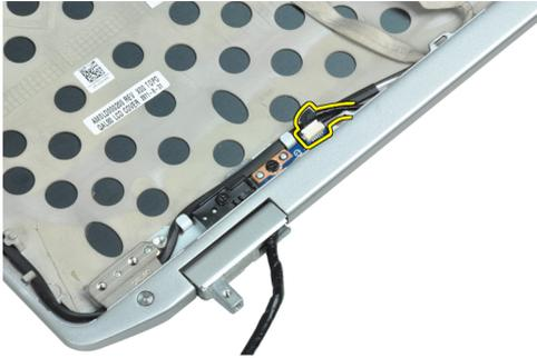
4. Remove the screw securing the power LED board to the display assembly.
