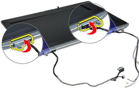
4. Pry loose the edge of hinge cap from the hinge and remove the hinge caps from the display assembly.
