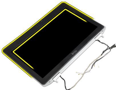
5. Remove the display bezel from the display assembly.
