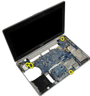
11. Gently lift the left edge of the system board assembly and raise it to a 45-degree angle and release the system board from the port connectors on the right.
