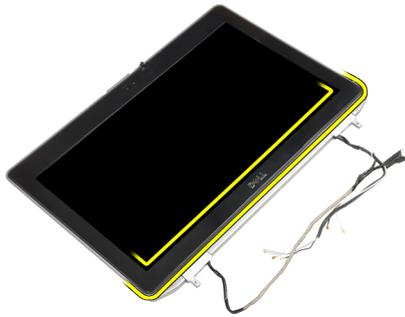
4. Pry up the left, right and top edges of the display bezel.
