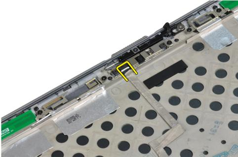
4. Peel back the adhesives securing the LVDS and camera cable to the display assembly.
