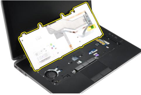
8. Peel back the adhesive tape securing the keyboard connector.
