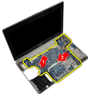
12. Release the system board from the connector port on the back and remove the system board from the system.
