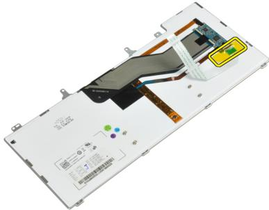
9. Remove the keyboard cable from the keyboard.
