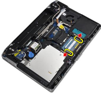
4. Remove the memory module from its connector on the system board.
