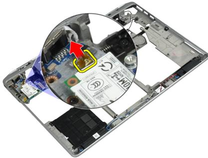
4. Remove the modem cable from the routing channel.
