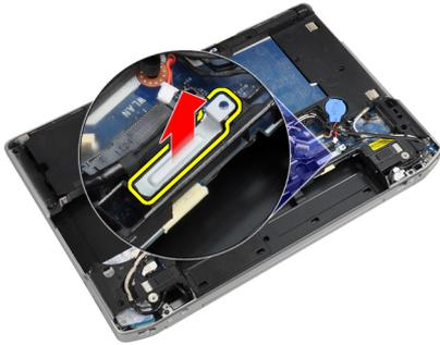
7. Disconnect the LVDS cable from the back of the system board.
