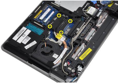
5. Remove the heat sink from the computer.
