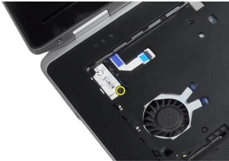
4. Pull out the tab from underneath the palmrest assembly.
