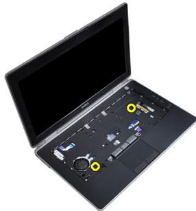
5. Disconnect the LED cable from the system board.
