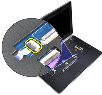
7. Disconnect the SD card cable from the system board.
