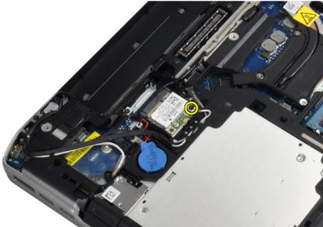
5. Remove the WLAN card from its slot on the system board.
