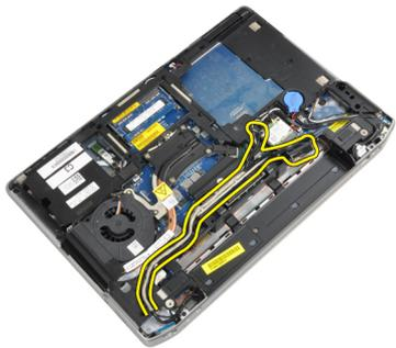
8. Disconnect any antennas connected to wireless solutions.
