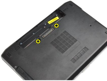
4. Remove the screws that secure the keyboard to the palmrest assembly.
