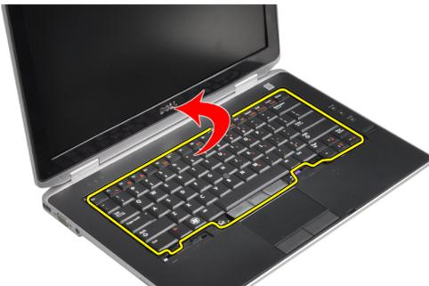
6. Disconnect the keyboard cable from the system board.
