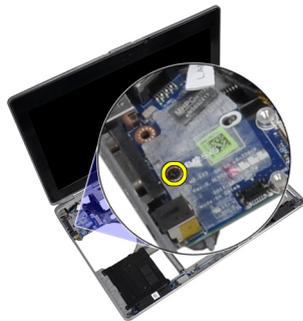
4. Remove the I/O board from the computer.
