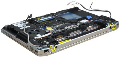
11. Remove the display assembly from the computer.
