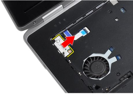
6. Hold and remove the modem card from the computer.
