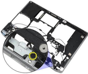
6. Remove the modem-connector bracket from the computer.
