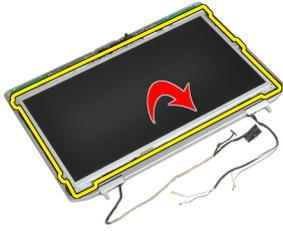
5. Peel off the LVDS cable connector tape and disconnect the LVDS cable from the display panel.
