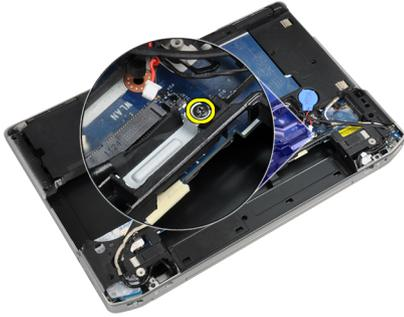
6. Remove the LVDS cable bracket from the computer.
