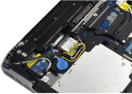
4. Remove the screw that secures the WLAN card to the computer.
