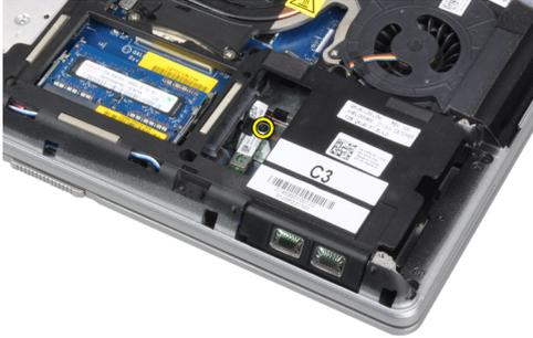
4. Lift up the card along the bottom edge and remove it from the housing.
