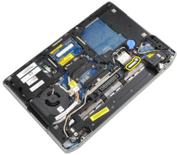
5. Pull upwards on the tab to disconnect the LVDS cable from the computer.
