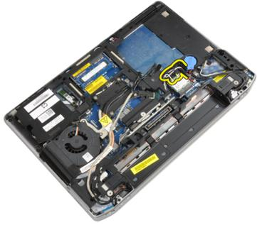
9. Remove any antennas from the routing channel.
