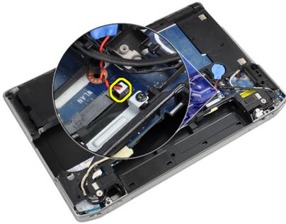
4. Disconnect the camera cable from the base of the system board.
