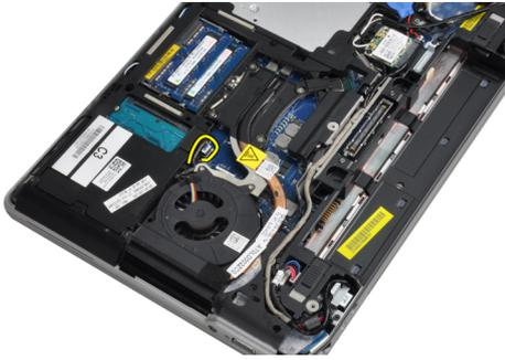
4. Remove the screws that secure the heat sink to the system board.
