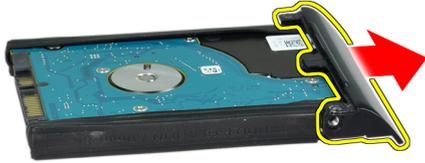
7. Remove the hard-drive isolation from the hard drive.
