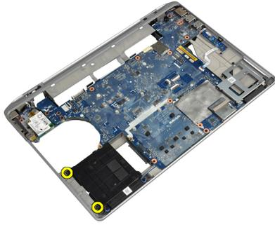
4. Lift the hard-drive support plate from the computer.
