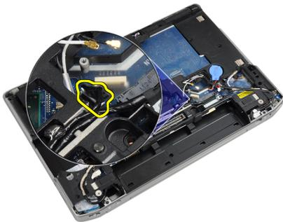
5. Remove the screw securing the LVDS cable bracket.
