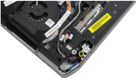
5. Remove the power-connector bracket from the computer.
