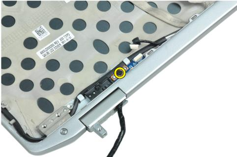
5. Remove the power LED board from the display assembly.
