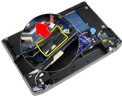
8. Disconnect the speaker cable from the base of the system board.
