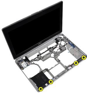
4. Remove the speaker cable from the routing channel.
