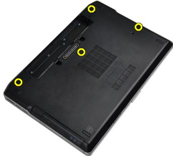
3. Lift the base cover to remove it from the computer.
