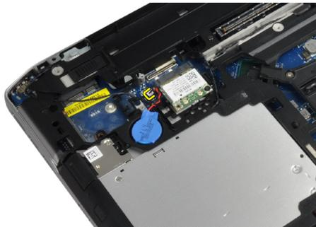
4. Pry the coin-cell battery upward and remove it from the computer.
