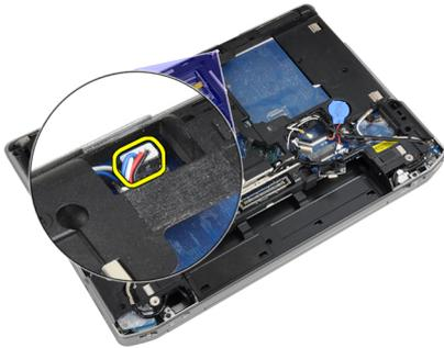
9. Flip the system over and disconnect the media board cable from the system board.
