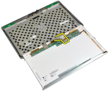
6. Remove the display panel from the display assembly.
