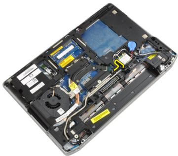
7. Remove the LVDS and camera cable from the routing channel.
