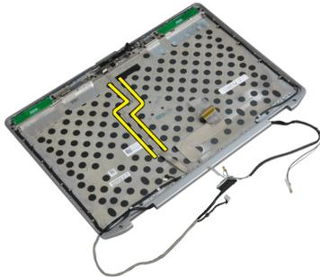
5. Remove the LVDS and camera cable from the display assembly.
