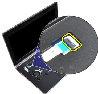
6. Disconnect the touchpad cable from the system board.
