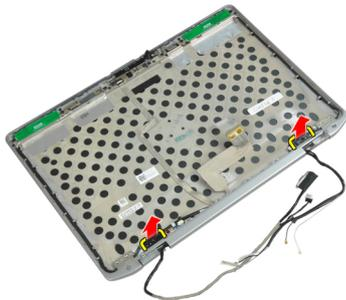
5. Remove the screws that secures the display hinges to the display assembly.
