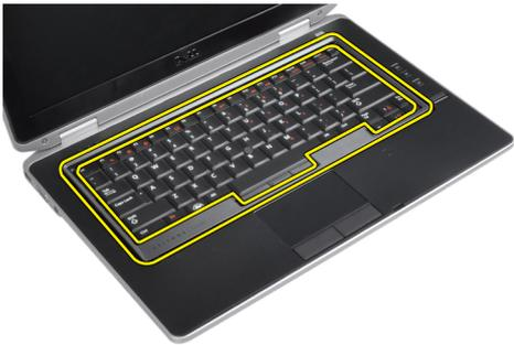
5. Lift up to remove the keyboard trim from the unit.
