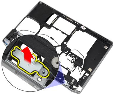
7. Remove the modem connector from the computer.
