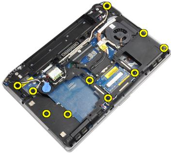
4. Flip the computer over and remove the screws that secure the palmrest assembly to the computer.
