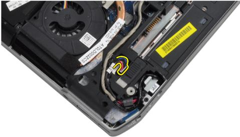
4. Remove the screw that secures the power-connector bracket to the computer.
