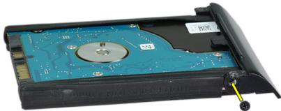
6. Remove the hard-drive caddy from the hard drive.
