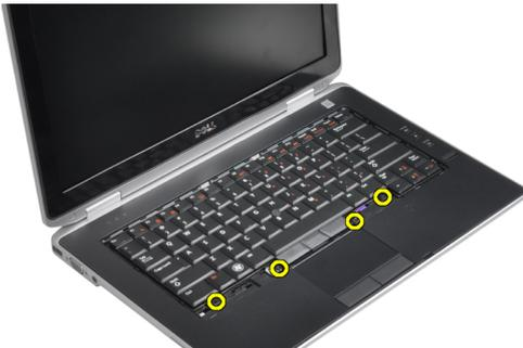
5. Lift and turn the keyboard to access the keyboard cable.
