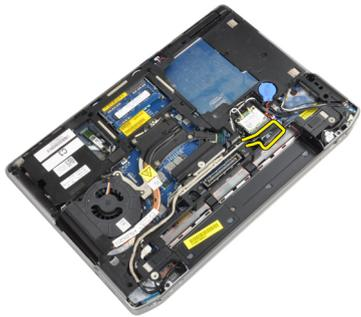
6. Disconnect the camera cable from the computer.
