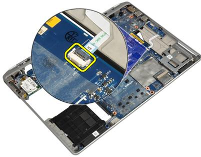
4. Remove the screws that secure the media board to the computer.
