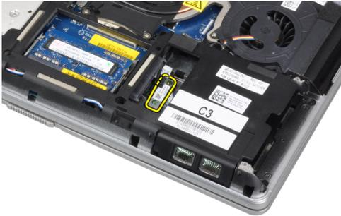
5. Disconnect the bluetooth cable from the system board and remove the card from the computer.
