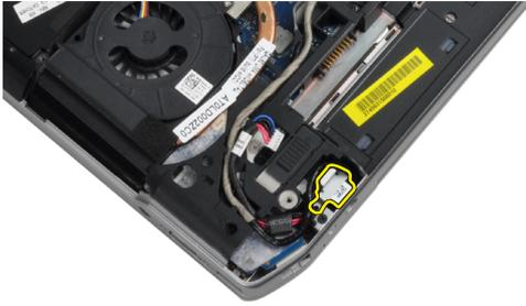
6. Remove the power-connector cable from the computer.
