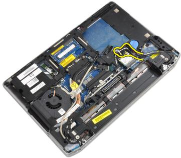
10. Remove the screws that secure the display assembly to the computer.
