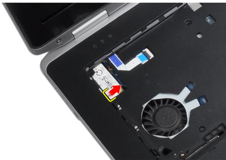
5. Use the tab and pull the lower right edge of the modem card from the slot.
