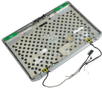
4. Remove the display hinge plates.
