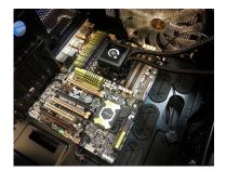
**6.** Install the graphics card into the x16 PCI Express slot and ensure the appropriate power connectors are used.
