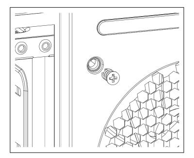
Assemble Fan by screw-down 4 fixing screws through the case mounting holes and the fan.
