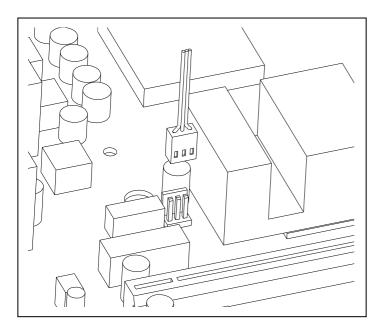
Connect the 3-Pin power connector to motherboard.
