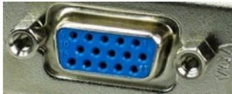
This 15-pin D-Sub output port is a very common sight. It is responsible for connection to CRT monitors and LCD monitors that support analog input. Digital signals must go through RAMDAC conversion before being sent through the D-Sub port as it is capable of only analog input.
