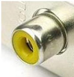
Also known as the AV or composite video connector, the RCA port is seen on home electronic devices including television sets and video cassette recorders. AV output is separated into one video and two audio signals (left and right channel). The yellow connector is often responsible for the video signal.
