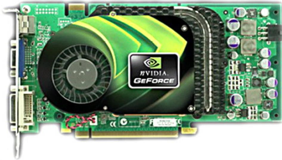
The EVGA e-GeForce 6800 GS follows NVIDIA's prescribed reference frequencies. As already mentioned above, the core clock is 425MHz and the Video RAM data rate is 1000MHz. Furthermore, the card has 256MB Video RAM, which is definitely sufficient for a card occupying the mid-range market.
