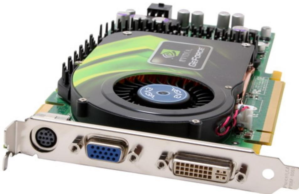
Like most VGA cards, there is a mainstream combination of S-Video, DVI-I and VGA ports on the rear bracket of the EVGA e-GeForce 6800 GS. A dual DVI-I combination would look more advanced than the common DVI-I + VGA setup, but the latter solution is a better fit for the card's target audience. Besides, the S-Video out port supports high resolution HDTV output, and serves as a future-proofing feature as HDTV is growing in popularity and is slated to one day replace traditional TV.
