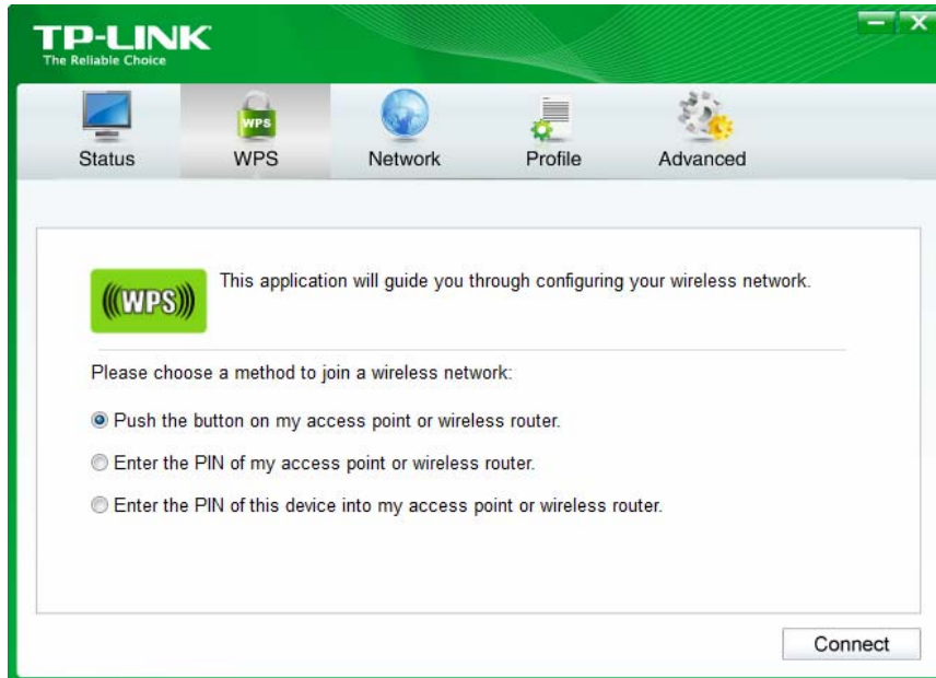
The WPS Configuration Screen of Wireless Adapter
