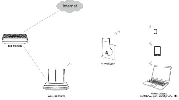
Figure 2-1 Typical connection of TL-WA854RE
