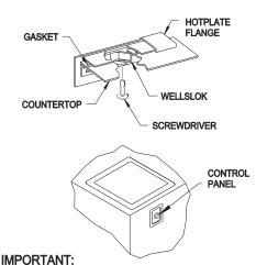
MOUNT APPLIANCE SO THAT THE CONTROL PANEL IS LOCATED TO THE FRONT OF THE FIXTURE.
