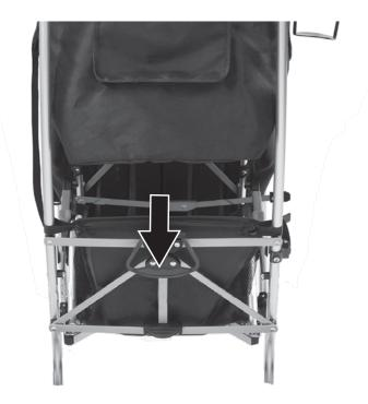
align rear wheels and push onto frame
