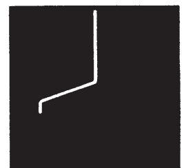
B-E paralleled by 680Ω
