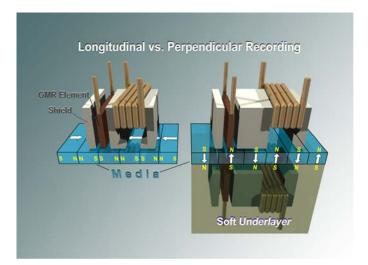
Seagate has demonstrated a recording areal density with perpendicular recording of 245 Gbpsi (Gigabits per square inch) with a data rate of 480 Mbits per second – more than double the 110 Gbpsi used in today's highest areal density disc drives – and 500 Gbpsi, which will increase the capacity of today's drives 5-fold, is possible with the new technology.
