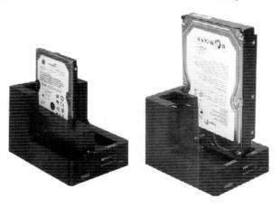
Connect the power supply to the mains.Connect the docking station to your computer USB port. Put the rear power switch in ON position.
