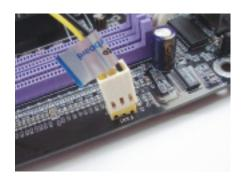
3. Connect the 3-pin connector of the fan cable assigned with a yellow and a black cable to the CPU fan motherboard connector.
