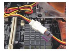
2. Connect the fan cable with 3 pin connector to the FAN Controller Cable
