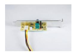
Connect the 3-pin connector with the yellow/red/black cable to the Controller Circuit board
