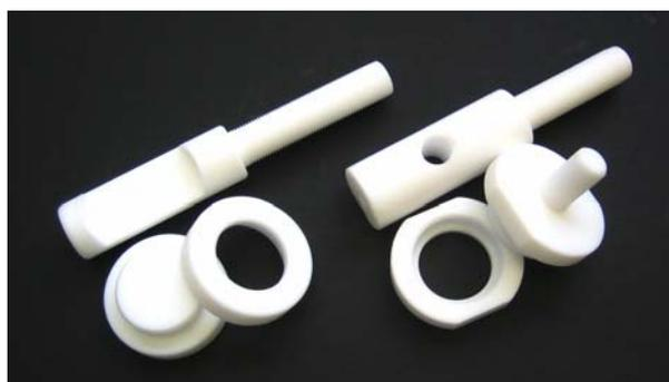
Fig. 30: Teflon disc holders from Tracerlab (l) and the improved disc holder (r).
