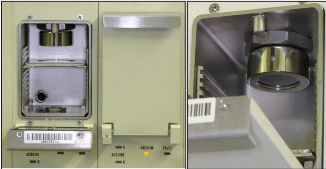
**Fig. 6:** An open alpha counting chamber next to a closed one (l). Semiconductor detector (*Canberra Model A300-17AM Alpha PIPS Detector*) (r) with the active surface facing downwards (PIPS = passivated implanted planar silicon).
