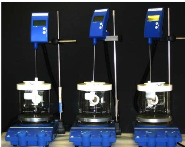
Fig. 29: Three sets of spontaneous deposition equipment
