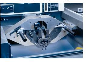
THE ML-5000 CAN ALSO BE EQUIPPED WITH FIXTURES DESIGNED FOR YOUR APPLICATION, SUCH AS THE GIMBAL/POCKET FIXTURE.
