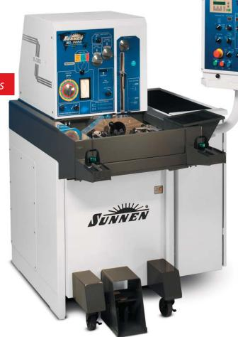
Sunnen Power Stroking assures constant stroke length and stroke rates. Combined with Automatic Size Control and a patented Dual Feed Pressure system, this means better control of bore size, finish and geometry than ever before – at high-production rates.
