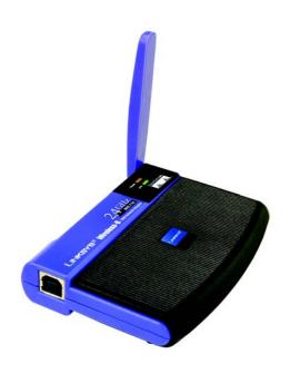
Connect your USB-equipped desktop or notebook computer to a wireless network with the Linksys Wireless-B USB Network Adapter, without the trouble of opening up the case of your desktop computer.
