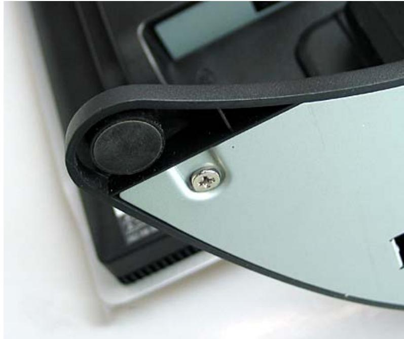
While the base stand has limited features, the detail and workmanship are very good. With the monitor stood on its side, we discover three rubber "feet" to provide more friction that will stop the monitor from moving unnecessarily.
