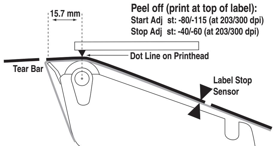
A special case is tickets with black marks. It is recommended to place the black mark adjacent to the perforation or the intended tear-off line. If the black mark is placed further down the media, this must be compensated for by a negative Stop Adjust setting.
