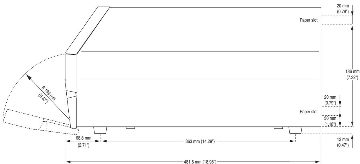
An optional paper cutter increases the printer's total length by 28 mm (1.1 inches).
