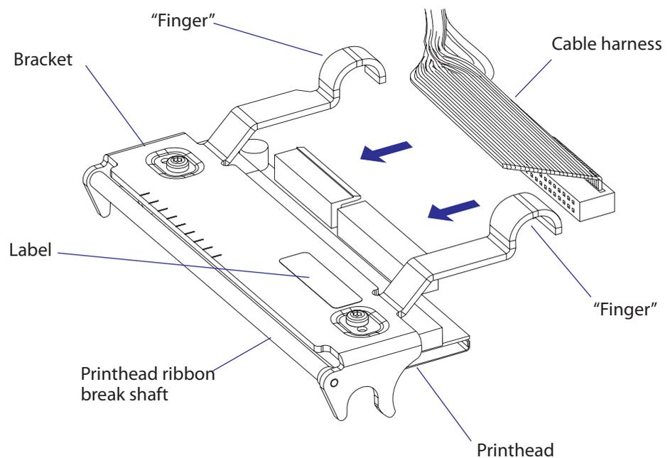
*Illustration shows the printhead of an EasyCoder PX4i.
