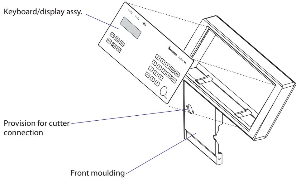
At the top part of the front moulding, there is a cavity for the keyboard/display assy. This assembly is affixed using two 2 mm hexagon grub screws underneath the keyboard part of the front moulding.
