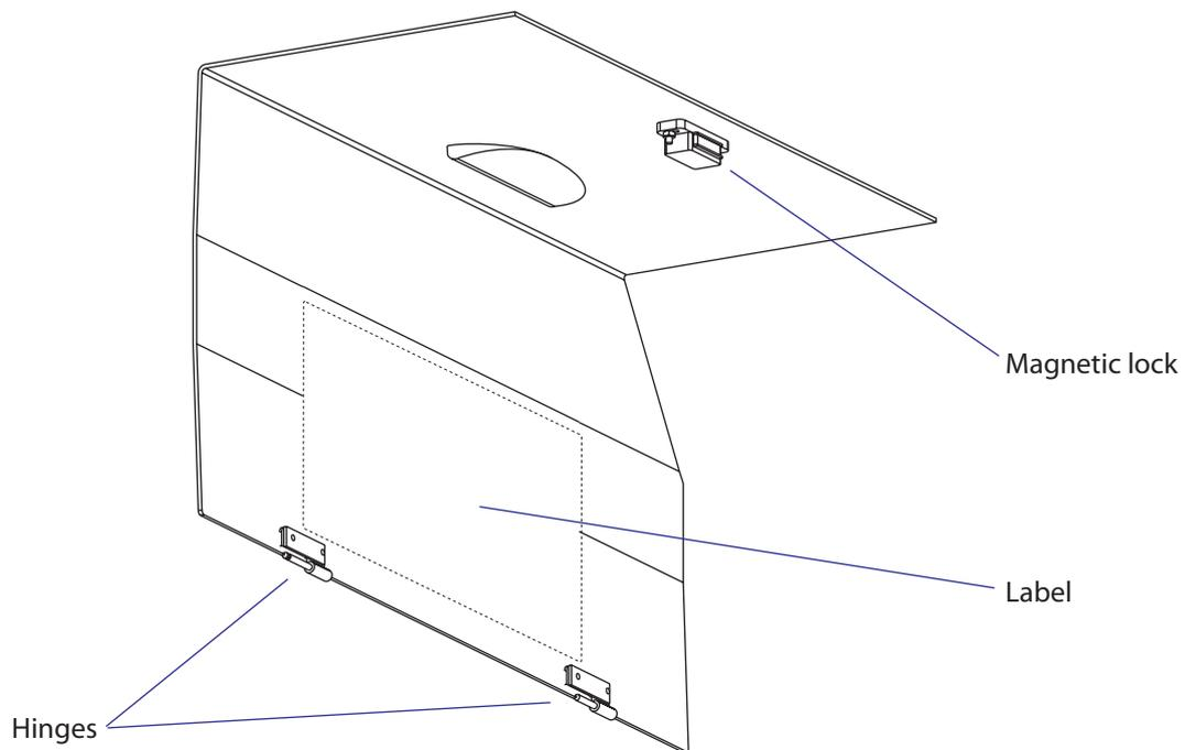
*Illustration shows the right-hand door of an EasyCoder PX4i. The door of the EasyCoder PX6i has a wider top part.*
