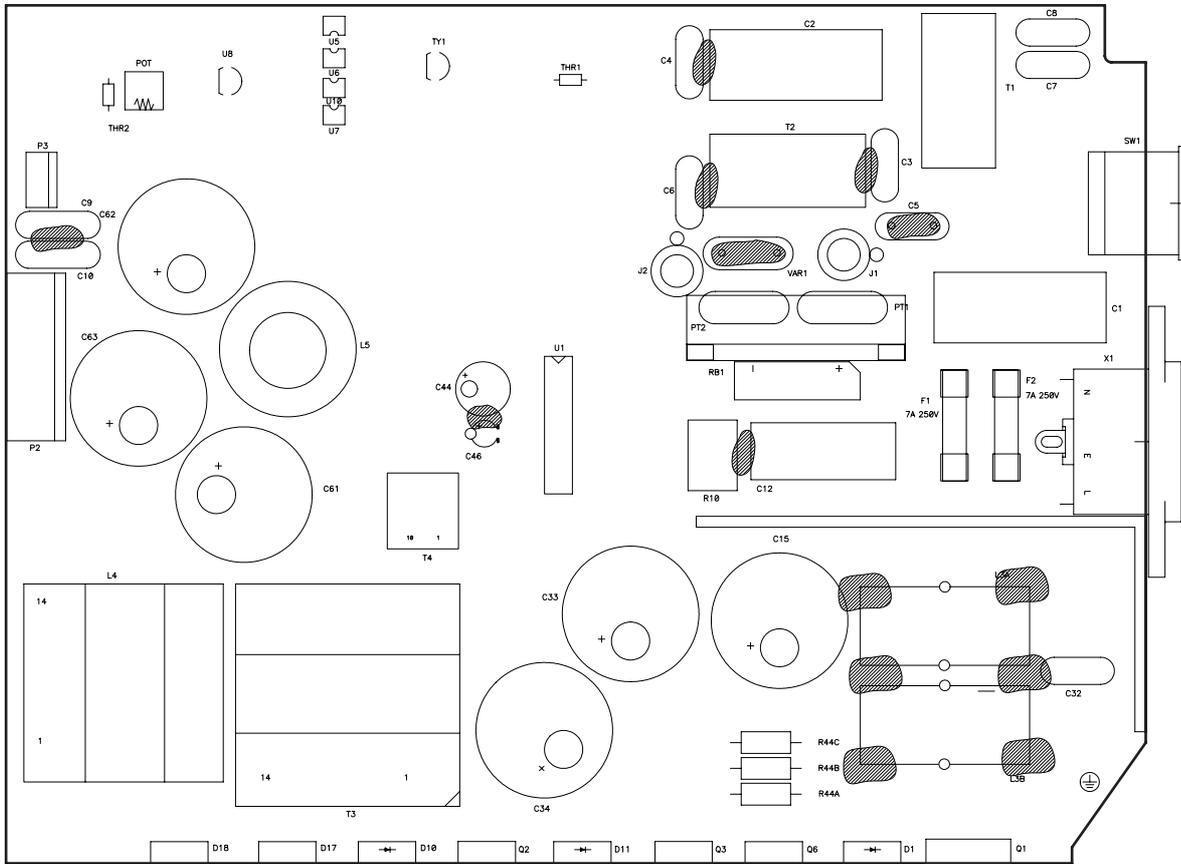
1-971632-25 Power Supply Unit; Component side
