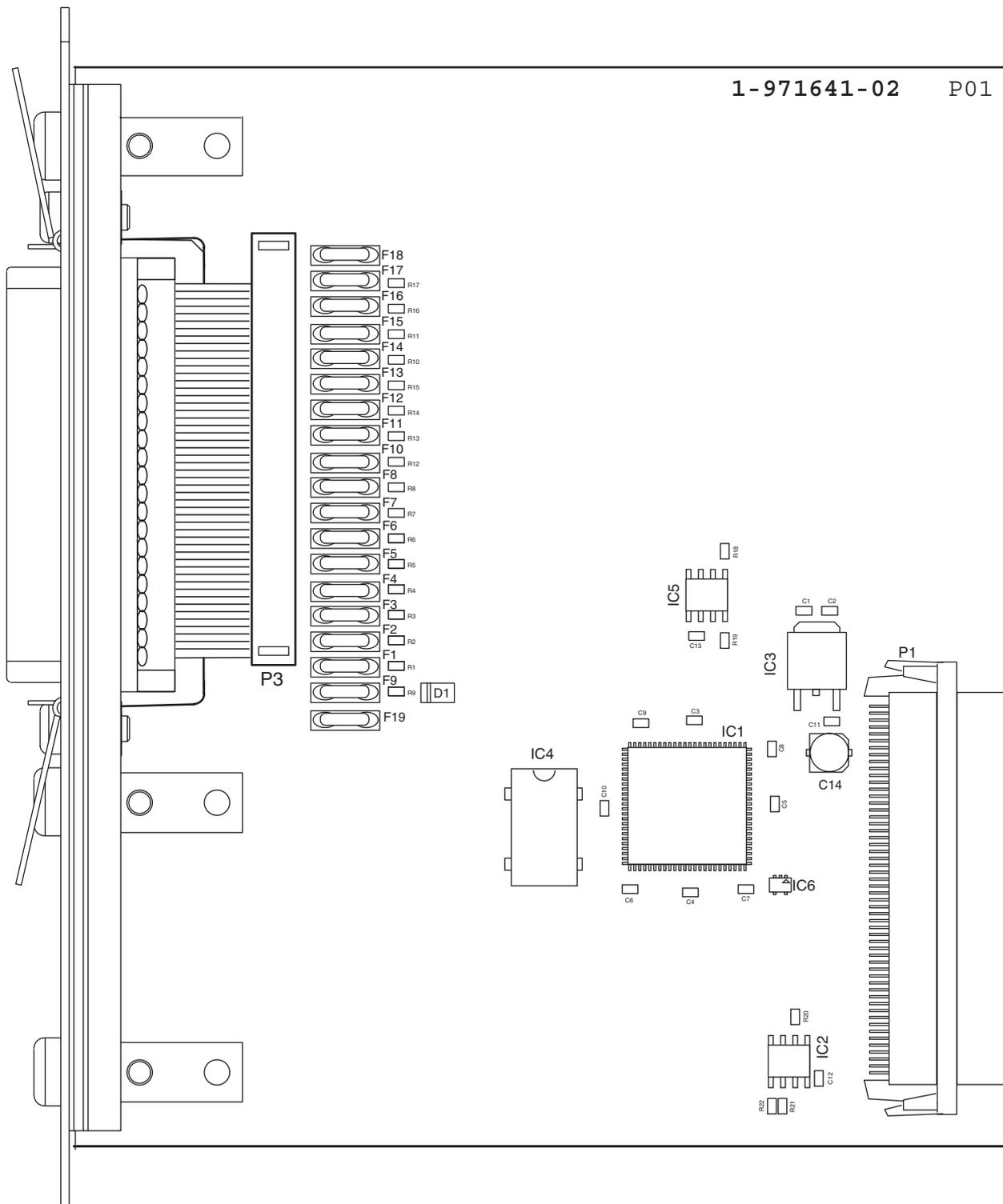
1-971641-27 IEEE 1284 Parallel Interface Board; Component side
