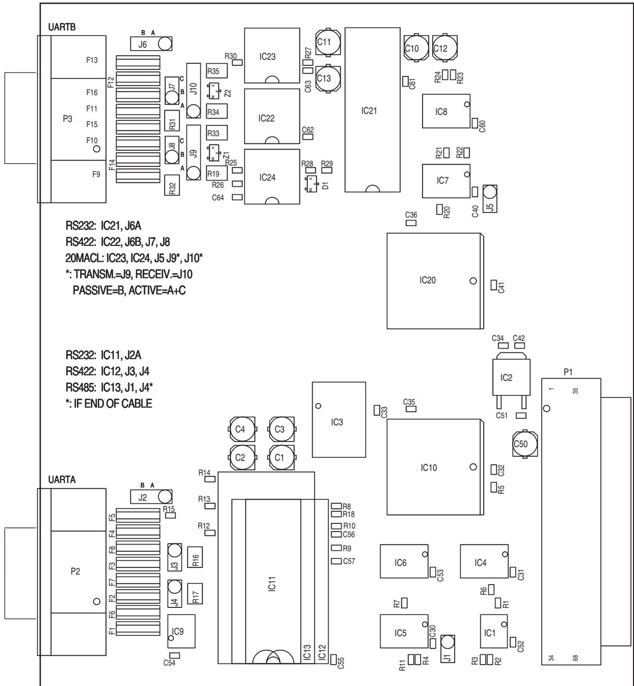
1-971642-26 Double Serial Interface Board; Component side
