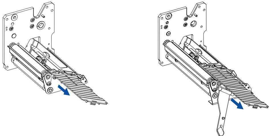
When cleaning the guide plates, use a soft cloth moistened with isopropyl alcohol. Do not use any other type of chemicals. Blow the sensors free from dust.
