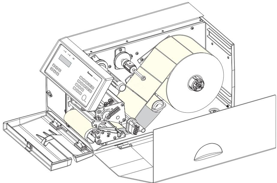
The batch takeup unit can accommodate approximately 1/4 to 1/3 of a full label roll depending on media thickness.
