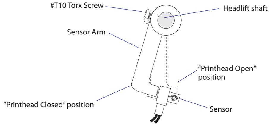
In Fingerprint, run this program which assists you in adjusting the headlift sensor arm:
