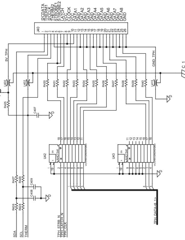
1-971630-26 CPU Board; Thermal Printhead Interface (Schematics #4)
