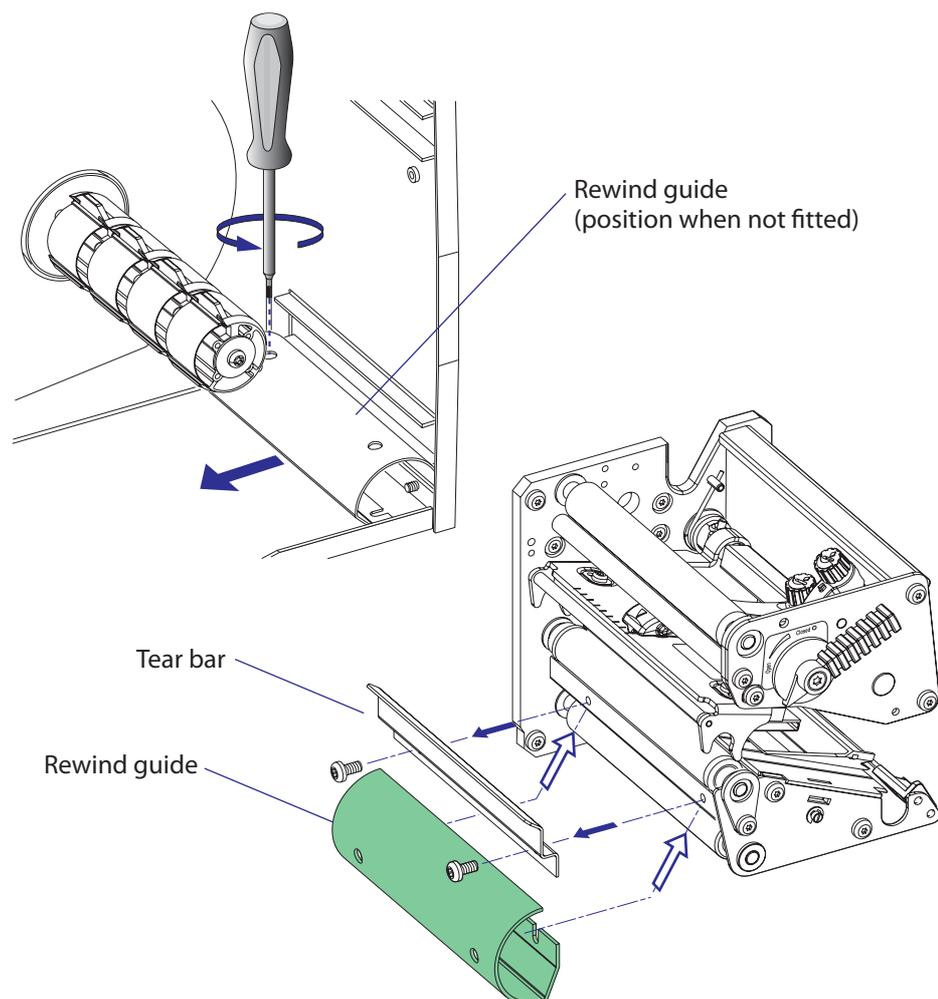
*The batch takeup guide plate is only used in EasyCoder PX4i.*
