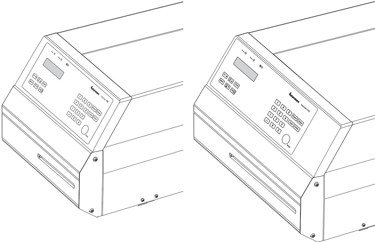
The cutter is intended to cut through continuous non-adhesive paper strip or through the liner between labels. It must not be used to cut through any kind of adhesive or other soft material, that may stick to the cutting parts and render the cutter inoperable or even damage the electric motor.
