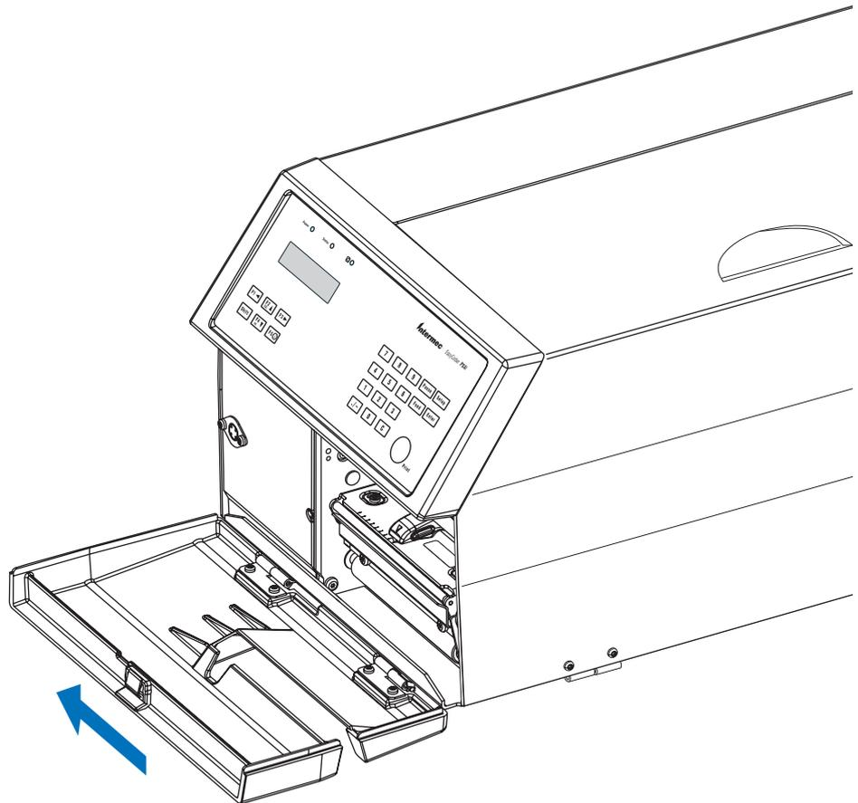
*The front hatch can be removed by pushing it to the left when open (illustration shows an EasyCoder PX4i).*
