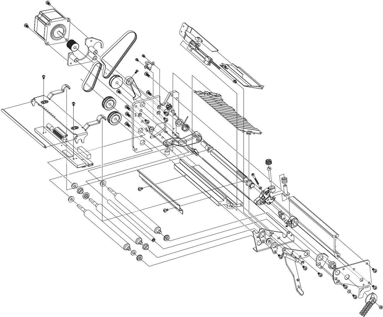
The parts of the print mechanism fitted inside the electronics compartment in an EasyCoder PX4i printer are illustrated below.
