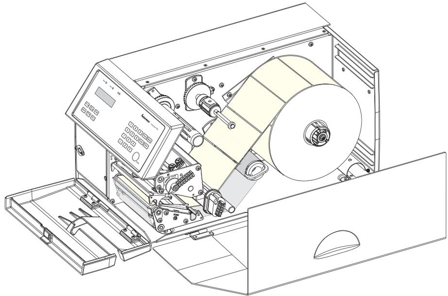
The liner takeup unit can accommodate the liner from a full roll of labels.
