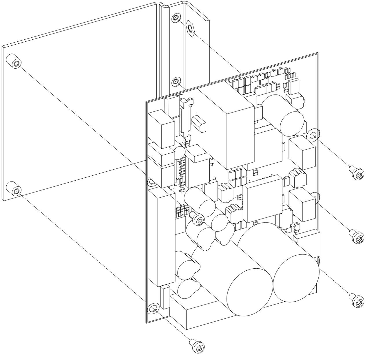
*The driver board and its attachment plate come as an assembled spare part.*
