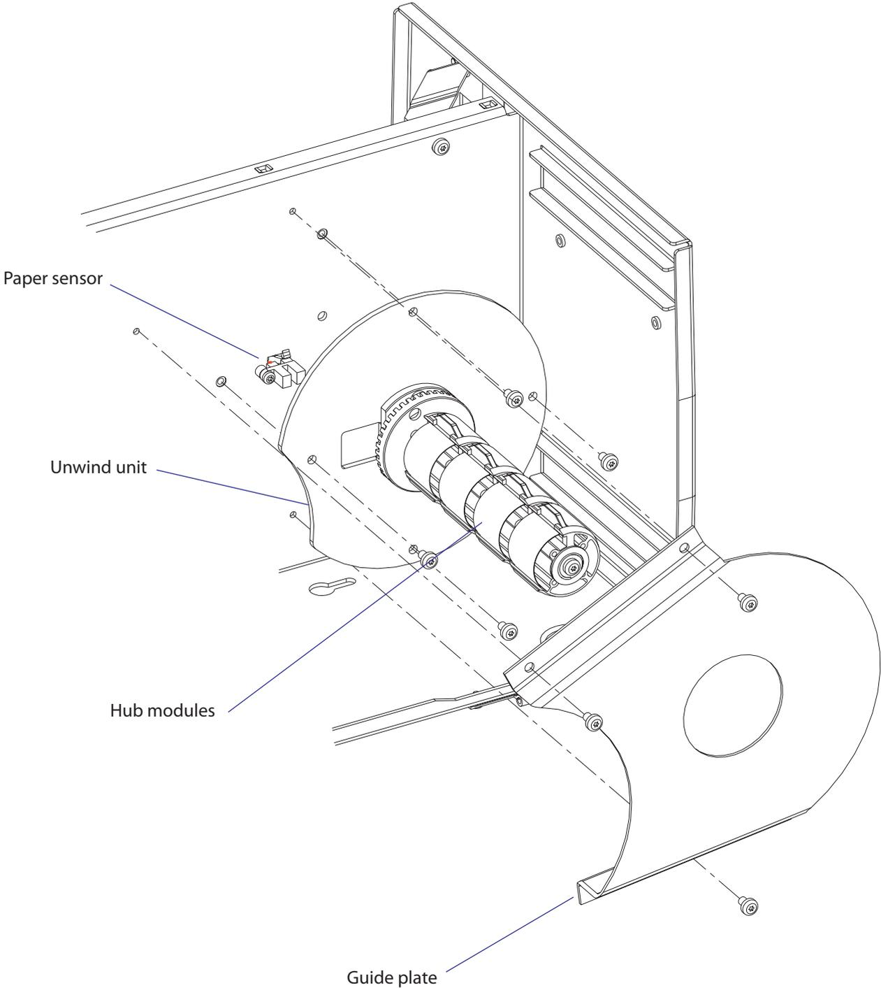
The media supply hub package can be dismantled by removing the #T20 Torx screw at the end of the shaft. Inside the outermost hub module, there is a spring that presses the hub package towards a felt pad in order to break the rotation. Else, the momentum of a large and heavy media roll might cause excessive media to be unwound when the printing is stopped. The brake torque should be  $70 \pm 20$  Nmm (see Appendix C).
