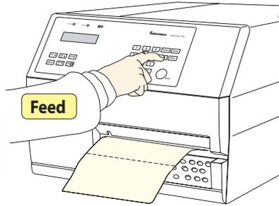
Press the Feed key to advance the media and adjust the media feed. Tear off the media by grabbing the outer edge and pull downwards.
