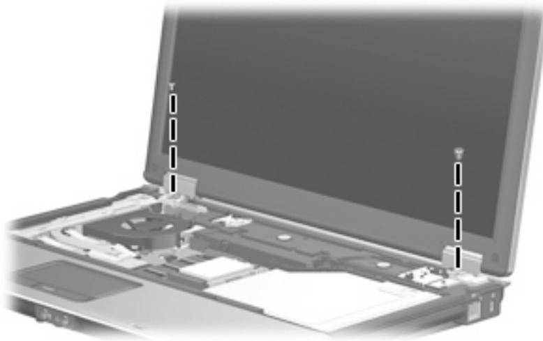
**Where used:** 2 screws that secure the display hinge covers to the computer
