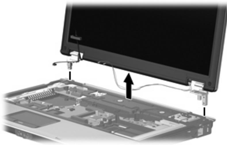
15. If it is necessary to replace the display bezel, display panel, or display hinges, remove the following:
