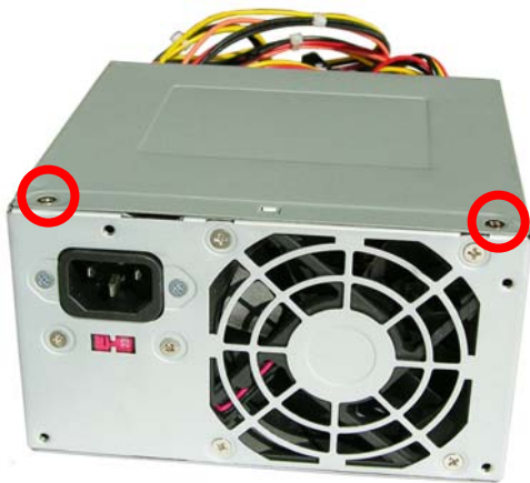
FIGURE 9: POWER SUPPLY 1: Power supply PCA screw locations
