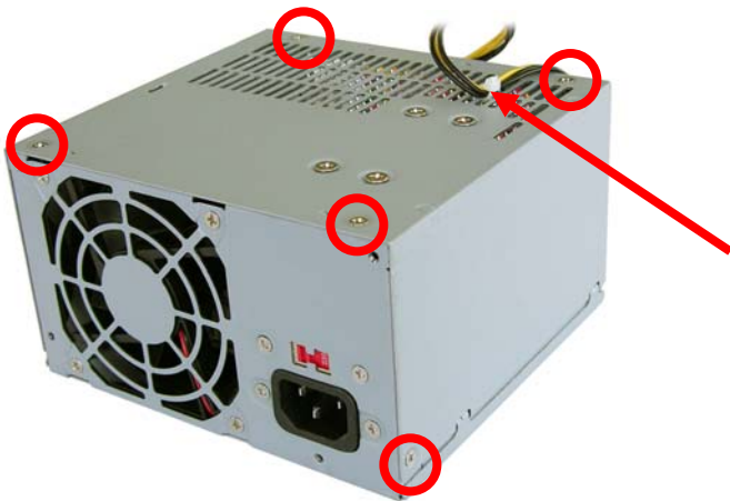
FIGURE 12: POWER SUPPLY 2: Plastic cable clamp and cover screw locations
