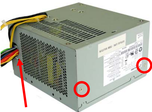
FIGURE 12: POWER SUPPLY 2: Plastic cable clamp and cover screw locations
