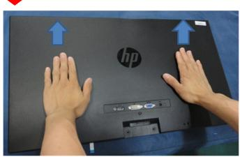
Step 4:Push up and disassemble the cover from the panel;
