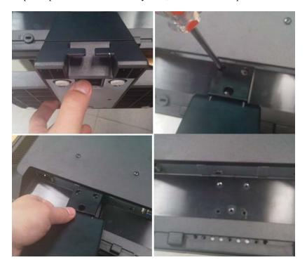
Step 2: Use tool to separate screw from rear cover, then separate rear cover from monitor head by hand.
