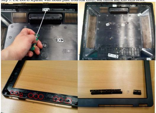
Step 9: Use tool to separate wall mount plate from rear cover, and button and lens form bezel.
