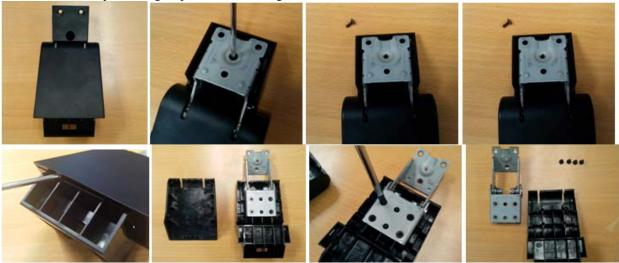
Step 11: Tear the rubber foot from base, then use tool to release screws from base plate, and use tool to separate base plate and base cover.
