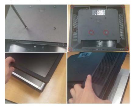
Step 3: Tear the tape from ctrl-BD wire, then disassemble the ctrl-BD wire, Separate panel and the bezel.
