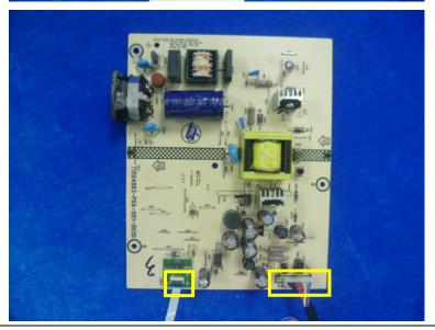
Remove the screws and disconnect the connectors to remove the MAIN BOARD and POWER BOARD.
