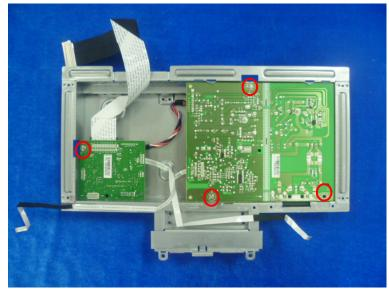
Remove the MAIN BOARD and POWER BOARD
