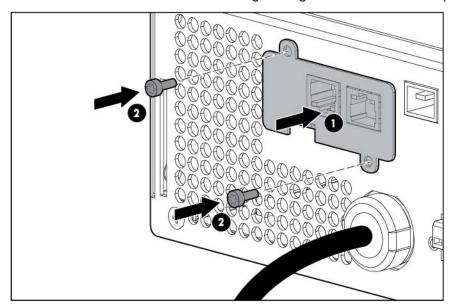
Secure the UPS Network Module using the two screws removed in step 1.
