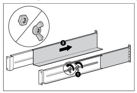
Insert screws through the rack into the mounting rail and the front of each mounting bracket.
