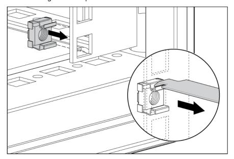
Insert screws through the mounting rail into the cage nuts or clip nuts.
