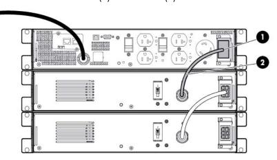
Attach the ERM connector bracket to the UPS as a cord retention bracket for the ERM cable.
