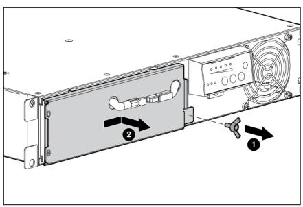
Remove the UPS battery modules.
