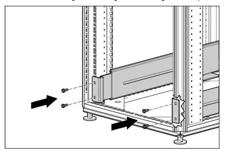
Tighten the wing nuts or hex nuts.
