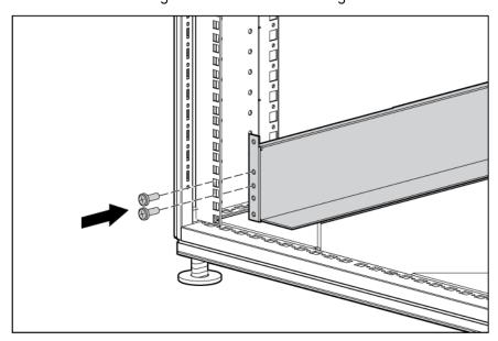
Install cage nuts or clip nuts into the rear of the rack.
