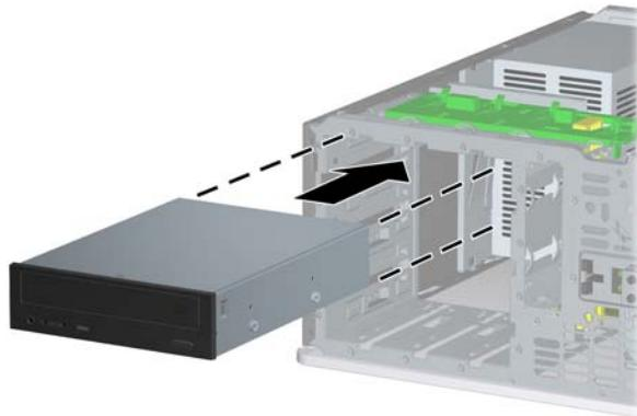
10. Gently slide the drive into the uppermost available bay until it snaps into place. When the drive is properly inserted, the drivelock will secure it. Repeat this step for each drive.
