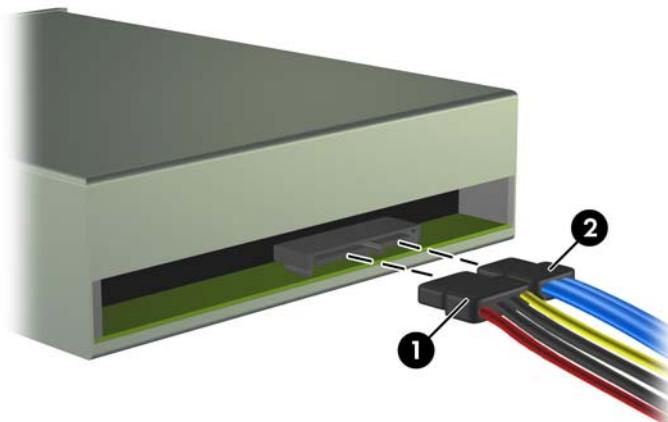
10. If you are installing a new drive, connect the opposite end of the data cable to the appropriate system board connector.
