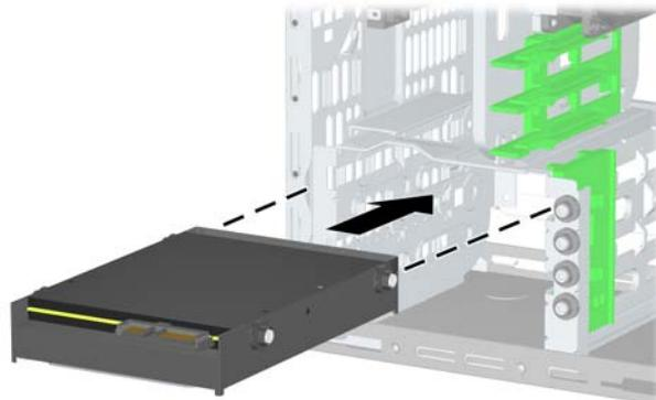
△ **CAUTION:** Make sure the guide screws line up with the guide slots in the drive cage. The use of unnecessary force when installing any drive into the drive bay may result in damage to the drive.
