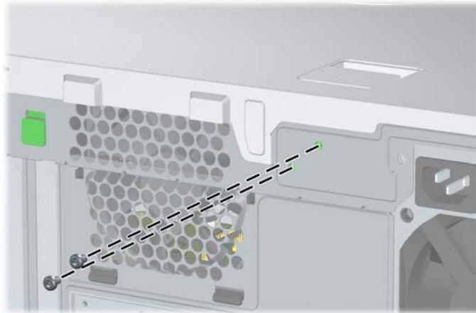
You can now remove the access panel. See [Removing the Computer Access Panel on page 11](#).
