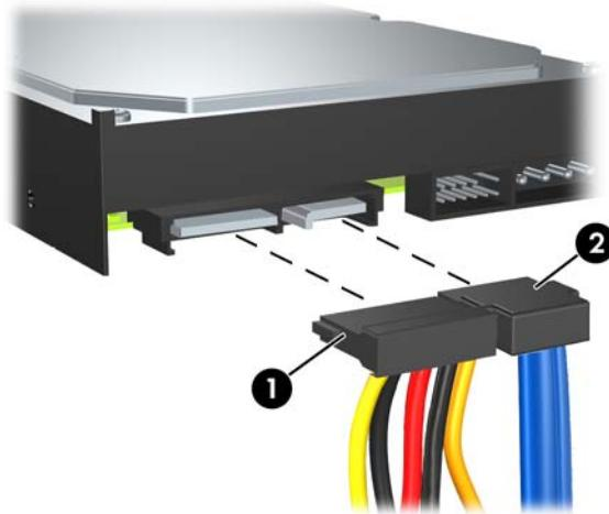
9. Connect the opposite end of the data cable to the appropriate system board connector.
