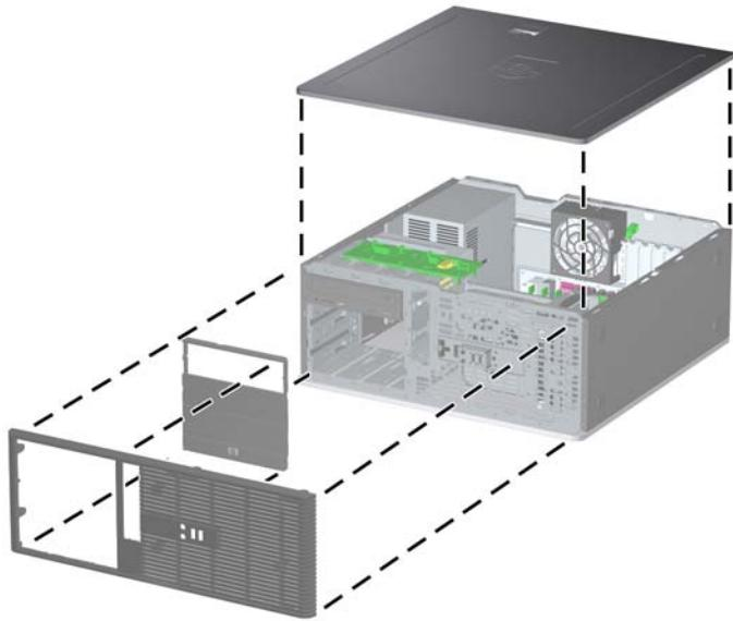
15. Replace the front bezel and computer access panel.
