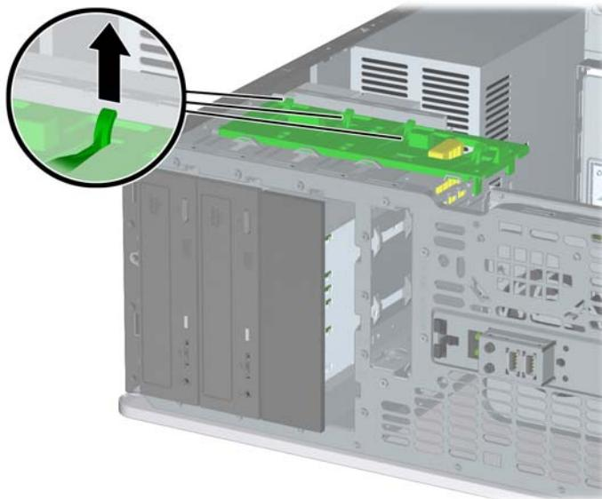
9. Before you reinstall each drive into the chassis, turn the drive so that it is perpendicular to the internal 3.5-inch drive. The drive should be parallel to the green latch drive bracket.
