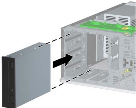
10. Gently slide the drive into the uppermost available bay until it snaps into place. When the drive is properly inserted, the drivelock will secure it. Repeat this step for each drive.
