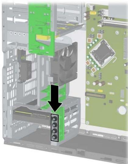
**Figure 2-24** Extra Optical Drive M3 Guide Screws Location
