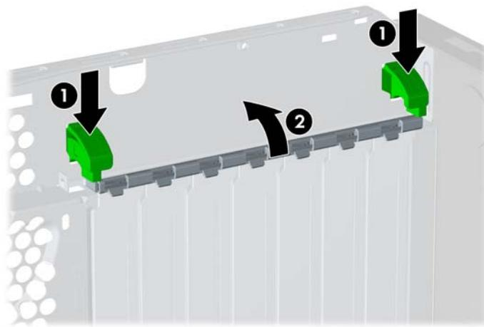
8. Before installing an expansion card, remove the expansion slot cover or the existing expansion card.
