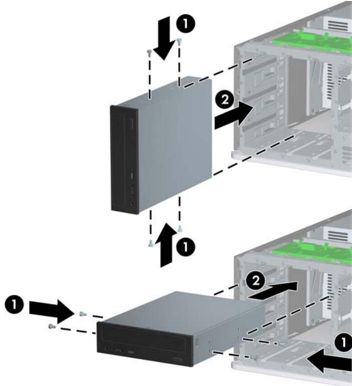
8. Install the drive in the desired drive bay by sliding it all the way into the front of the drive cage until it locks (2). The drivelock automatically secures the drive in the bay.
