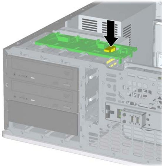
9. Before you reinstall each drive into the chassis, turn it so that it is in the same orientation as the internal 3.5-inch drive. The bottom of the drive should be parallel to the yellow drivelock.
