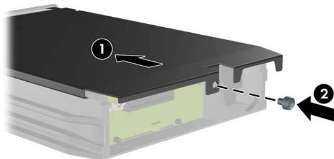
10. Slide the hard drive carrier into the enclosure on the computer and lock it with the key provided.
