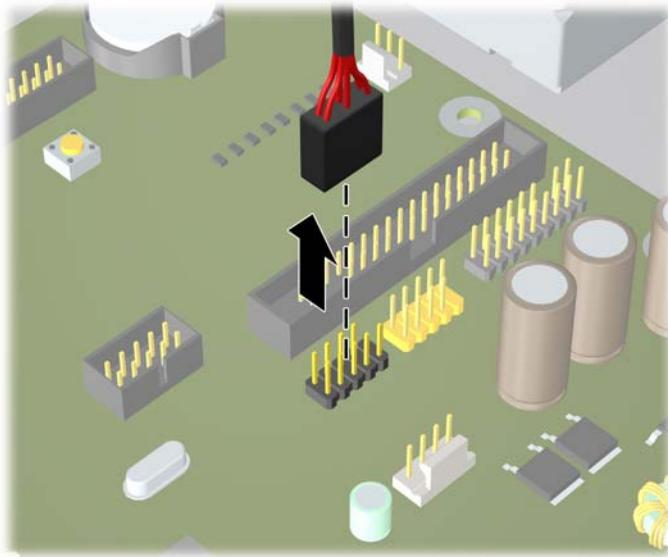
**Figure 2-19** Disconnecting the Media Card Reader 1394 Cable
