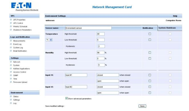
The environment sensor measures temperature, humidity and gives the status of the 2 contacts (used for door, alarms or generator unit).
