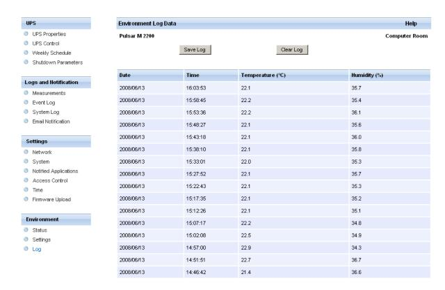
The two environment sensor measurements: Temperature and Humidity are recorded at an interval defined by the Environment log interval in the <u>System settings</u> page.
