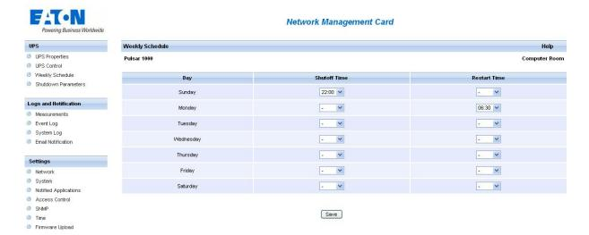
UPS configuration may prevent the shutdown and restart commands from being properly run. Read the UPS user manual for more information.
