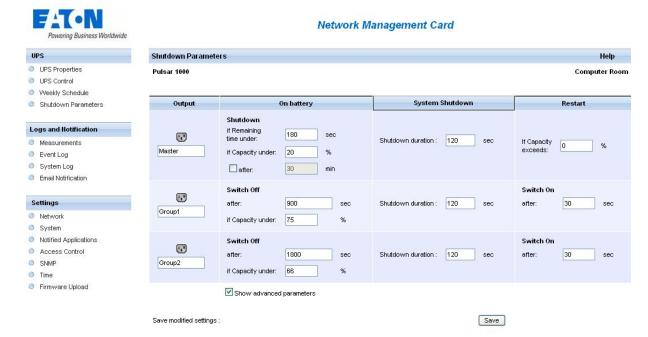
When you tick the **Show advanced parameters** option, extra parameters are displayed. These parameters enable, in particular, adjustment of certain thresholds related to the percentage of remaining battery charge level.
