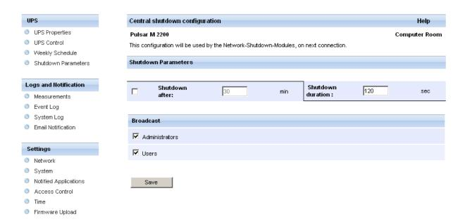
This page is used to define either the "shutdown" or the "notification" settings used by the Intelligent Power Protector that connects to Network Management Card. These settings are used by the Intelligent Power Protector if they are in central-configuration mode or if their configuration is not valid.
