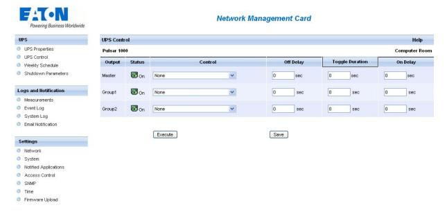
This page enables triggering of startup and shutdown sequences for the UPS main output and controlled outlets.
