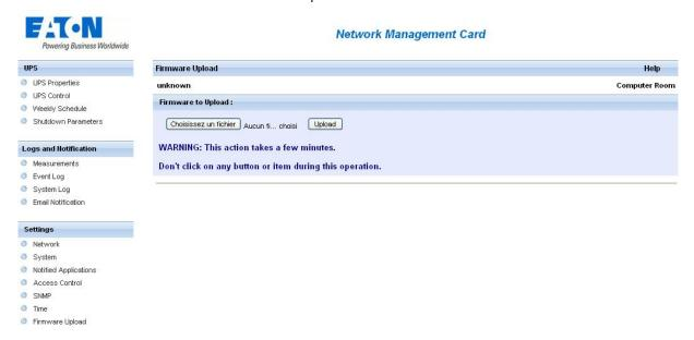
To upload a new version of the card's firmware, select the file to be loaded using the **Browse...** button and click Upload.
