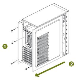
Unscrew to remove left and right panel.
