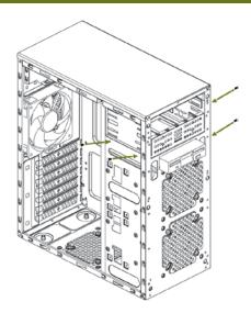
• Insert the external 3.5" device from the front panel into the chassis then secure with screws.
