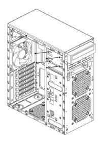
Insert the 5.25" device from the front panel into the chassis then secure with screw.
