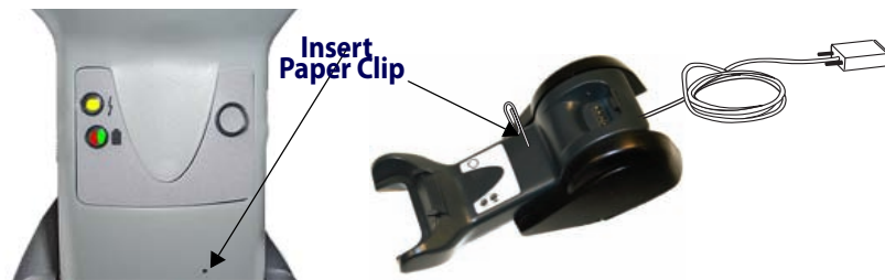
Figure 10. Disconnecting the Cable
