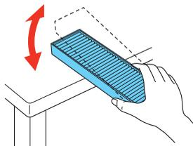
**Note:** Do not use excessive force when tapping the air filter, or it may crack and become unusable. Do not rinse the air filter in water, or use any detergent or solvent to clean it. Do not use canned air, or the gases may leave a residue.
