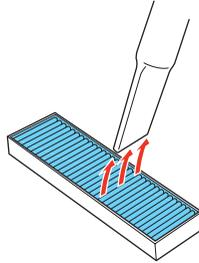
If the dirt is difficult to remove or the filter is broken, replace it. You can purchase air filter part number V13H134A38 from an authorized Epson reseller. To find the nearest reseller, please contact your nearest Epson authorized reseller or contact Epson as described in straight out on “Where to Get Help” on page 70.
