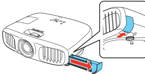
4. Remove the air filter as shown.
