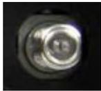
Current LCD TVs provide at least one RF connector to receive TV signals from an analog cable or antenna. Of course, the RF connector can be used to connect with some VCRs or game consoles as well. The RF connector also carries the audio signal, thus the connection is simple, meaning that there is no need to connect separate video and audio cables separately. On the LCD TV, the RF connector is often labeled as "Antenna", "CATV", or "TV-in".
